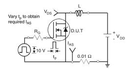
Fig. 12a - Unclamped Inductive Test Circuit
