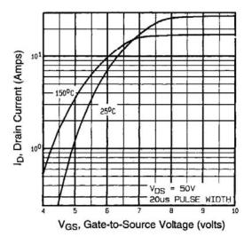
Fig. 3 - Typical Transfer Characteristics
