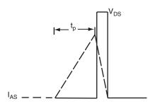
Fig. 12b - Unclamped Inductive Waveforms
