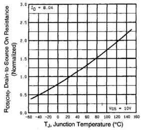
Fig. 4 - Normalized On-Resistance vs. Temperature
