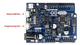
Either USB port can be used for programming the board, although using the Programming port is recommended due to the way the erasing of the chip is handled:
