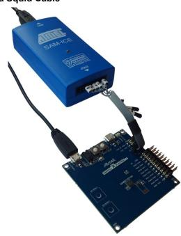
Figure 5-7. SAM-ICE using an Atmel-ICE Adapter
