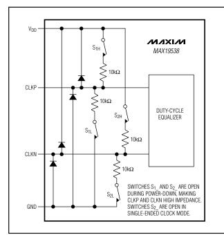
Figure 5. Simplified Clock Input Circuit
