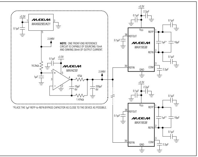
Figure 13. External Buffered Reference Driving Multiple ADCs
