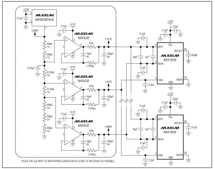
Figure 14. External Unbuffered Reference Driving Multiple ADCs
