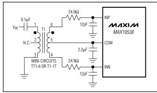
Figure 10. Transformer-Coupled Input Drive for Input Frequencies Up to Nyquist
