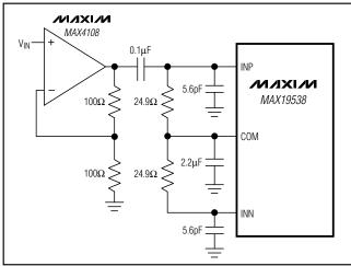
Figure 12. Single-Ended, AC-Coupled Input Drive
