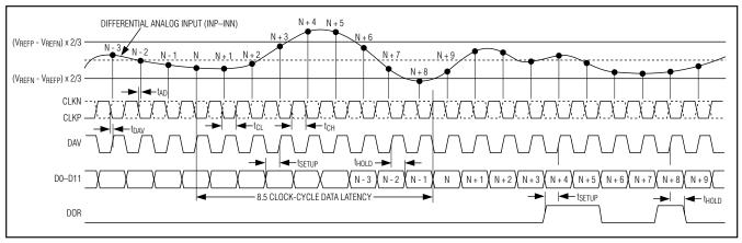
Figure 6. System Timing Diagram
