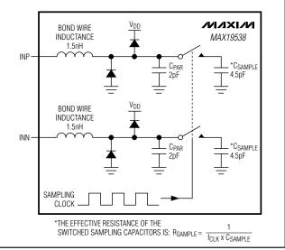
Figure 3. Simplified Input Track-and-Hold Circuit
