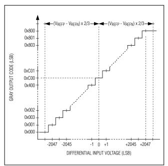
Figure 8. Gray-Code Transfer Function  $(G/\overline{T} = 1)$
