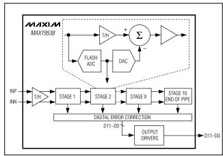
Figure 1. Pipeline Architecture—Stage Blocks
