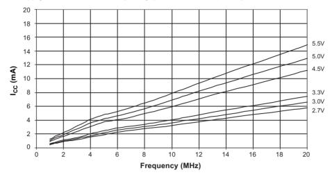
Figure 6-5. Idle Supply Current versus Frequency (1MHz to 20MHz), Temp = 125°C
