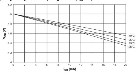
Figure 6-17. Output High Voltage versus Output High Current (V<sub>CC</sub> = 3V)
