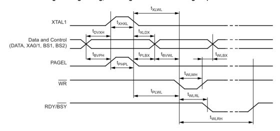
Figure 5-124. Parallel Programming Timing, Loading Sequence with Timing Requirements<sup>(1)</sup>
