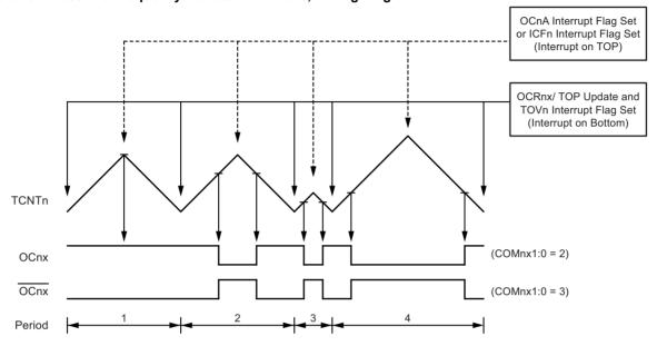
The Timer/Counter overflow flag (TOV1) is set at the same timer clock cycle as the OCR1x registers are updated with the double buffer value (at BOTTOM). When either OCR1A or ICR1 is used for defining the TOP value, the OC1A or ICF1 flag set when TCNT1 has reached TOP. The interrupt flags can then be used to generate an interrupt each time the counter reaches the TOP or BOTTOM value.
