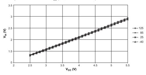
Figure 6-19. I/O Pin Input Threshold versus  $V_{\text{CC}}$  (VIL, I/O Pin Read as 0)
