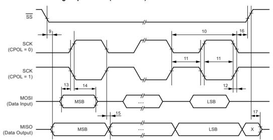
Figure 6-3. SPI Interface Timing Requirements (Slave Mode)
