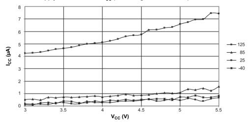
Figure 6-7. Power-down Supply Current versus V<sub>CC</sub> (Watchdog Timer Enabled)
