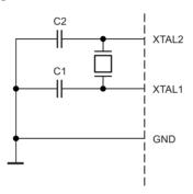
The low power oscillator can operate in three different modes, each optimized for a specific frequency range. The operating mode is selected by the fuses CKSEL3..1 as shown in Table 5-6.
