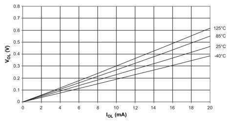
Figure 6-10. Output Low Voltage versus Output Low Current ( $V_{CC} = 3V$ )
