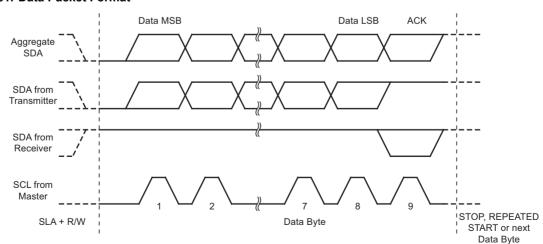
Figure 5-81. Data Packet Format
