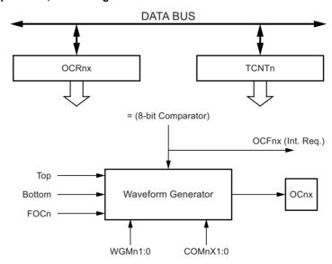
The OCR2x register is double buffered when using any of the pulse width modulation (PWM) modes. For the normal and clear timer on compare (CTC) modes of operation, the double buffering is disabled. The double buffering synchronizes the update of the OCR2x compare register to either top or bottom of the counting sequence. The synchronization prevents the occurrence of odd-length, non-symmetrical PWM pulses, thereby making the output glitch-free.
