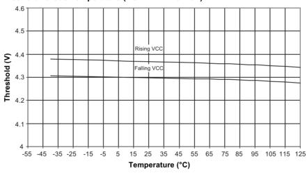
Figure 6-28. BOD Threshold versus Temperature (BODLEVEL is 2.7V)
