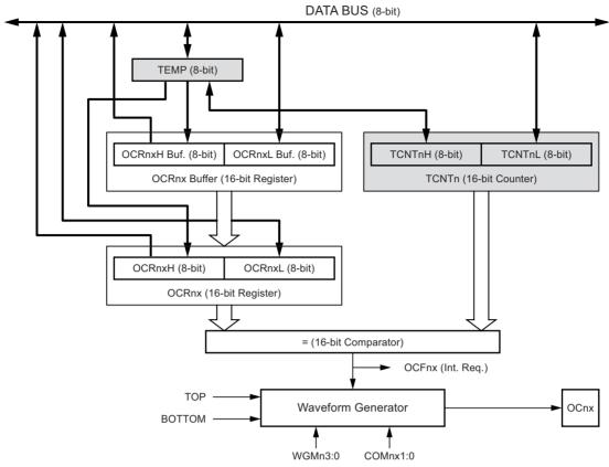
The OCR1x register is double buffered when using any of the twelve pulse width modulation (PWM) modes. For the normal and clear timer on compare (CTC) modes of operation, the double buffering is disabled. The double buffering synchronizes the update of the OCR1x compare register to either TOP or BOTTOM of the counting sequence. The synchronization prevents the occurrence of odd-length, non-symmetrical PWM pulses, thereby making the output glitch-free.
