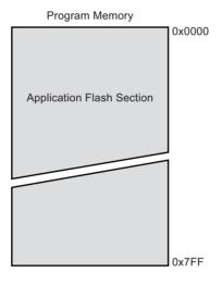
Figure 5-8. Program Memory Map, Atmel ATA6612C/ATA6613C
