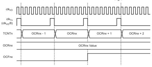
Figure 5-63 shows the setting of OCF2A and the clearing of TCNT2 in CTC mode.
