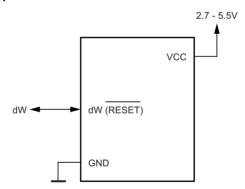
Figure 5-113 shows the schematic of a target MCU, with debugWIRE enabled, and the emulator connector. The system clock is not affected by debugWIRE and will always be the clock source selected by the CKSEL fuses.
