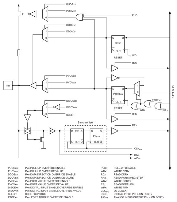
Note: 1. WRx, WPx, WDx, RRx, RPx, and RDx are common to all pins within the same port. clk<sub>I/O</sub>, SLEEP, and PUD are common to all ports. All other signals are unique for each pin.
