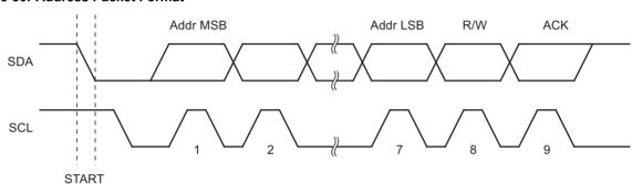
Figure 5-80. Address Packet Format
