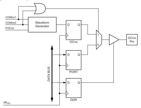
The general I/O port function is overridden by the output compare (OC2x) from the waveform generator if either of the COM2x1:0 bits are set. However, the OC2x pin direction (input or output) is still controlled by the data direction register (DDR) for the port pin. The data direction register bit for the OC2x pin (DDR\_OC2x) must be set as output before the OC2x value is visible on the pin. The port override function is independent of the waveform generation mode.
