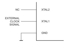
When this clock source is selected, start-up times are determined by the SUT fuses as shown in Table 5-16.
