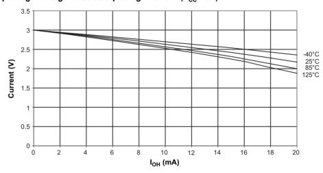
Figure 6-13. Reset Pull-Up Resistor Current versus Reset Pin Voltage ( $V_{CC} = 5V$ )
