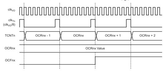
Figure 5-37 shows the setting of OCF0A and the clearing of TCNT0 in CTC mode and fast PWM mode where OCR0A is TOP.
