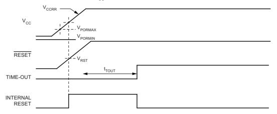
Figure 5-17. MCU Start-up, RESET Extended Externally
