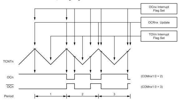
Figure 5-59. Phase Correct PWM Mode, Timing Diagram
