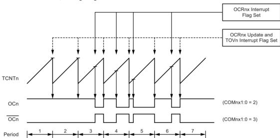
Figure 5-32. Fast PWM Mode, Timing Diagram
