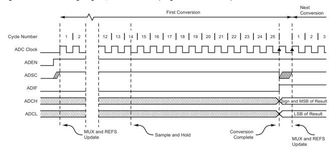
Figure 5-104. ADC Timing Diagram, Single Conversion
