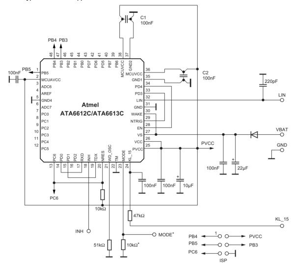
$<sup>^{\</sup>star}$  The MODE pin can be connected directly to GND, if it is not needed to disable the Watchdog
