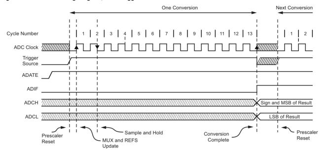
Figure 5-106. ADC Timing Diagram, Free Running Conversion
