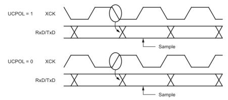
The UCPOLn bit UCRSC selects which XCKn clock edge is used for data sampling and which is used for data change. As Figure 5-71 shows, when UCPOLn is zero the data will be changed at rising XCKn edge and sampled at falling XCKn edge. If UCPOLn is set, the data will be changed at falling XCKn edge and sampled at rising XCKn edge.
