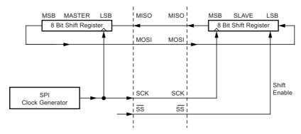
The system is single buffered in the transmit direction and double buffered in the receive direction. This means that bytes to be transmitted cannot be written to the SPI data register before the entire shift cycle is completed. When receiving data, however, a received character must be read from the SPI data register before the next character has been completely shifted in. Otherwise, the first byte is lost.
