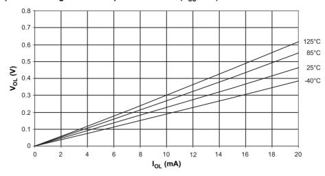
Figure 6-15. Output Low Voltage versus Output Low Current ( $V_{CC} = 3V$ )
