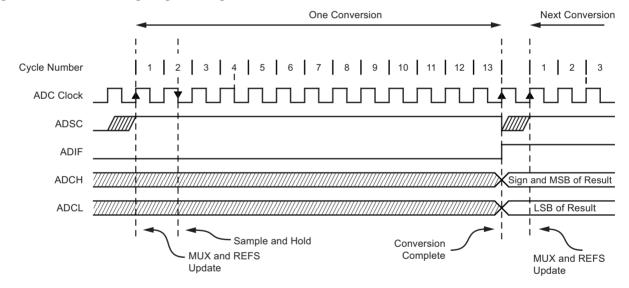
Figure 5-105. ADC Timing Diagram, Auto Triggered Conversion
