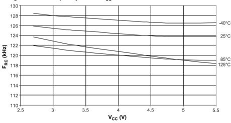
Figure 6-23. Calibrated 8MHz RC Oscillator Frequency versus Temperature
