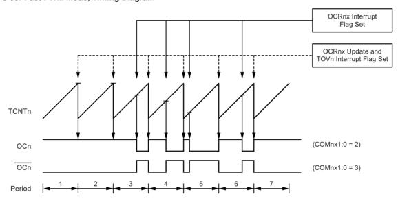
The Timer/Counter overflow flag (TOV2) is set each time the counter reaches TOP. If the interrupt is enabled, the interrupt handler routine can be used for updating the compare value.
