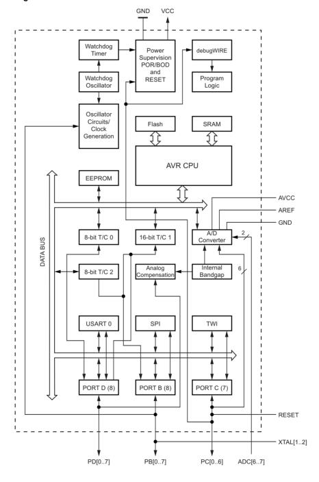
The Atmel® AVR® core combines a rich instruction set with 32 general purpose working registers. All the 32 registers are directly connected to the arithmetic logic unit (ALU), allowing two independent registers to be accessed in one single instruction executed in one clock cycle. The resulting architecture is more code efficient while achieving throughputs up to ten times faster than conventional CISC microcontrollers.
