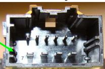
B. Begin mating procedure by sliding the receptacle connector assembly into the header assembly, press firmly until you hear an audible click.
