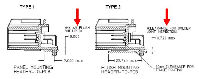
TYPE 1: THE BOTTOM STANDOFF RIBS ARE NOT USED. THE HEADER(S) RESTS FLAT ON
