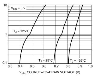
Figure 10. Diode Forward Voltage vs. Current
