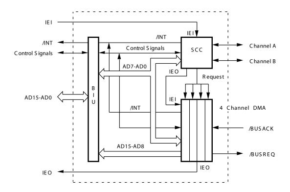
Figure 1. Z16C35 Functional Block Diagram
