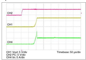
**Figure 1** — Inrush transient current at full load and 48  $V_{\rm IN}$  with PC enabled
