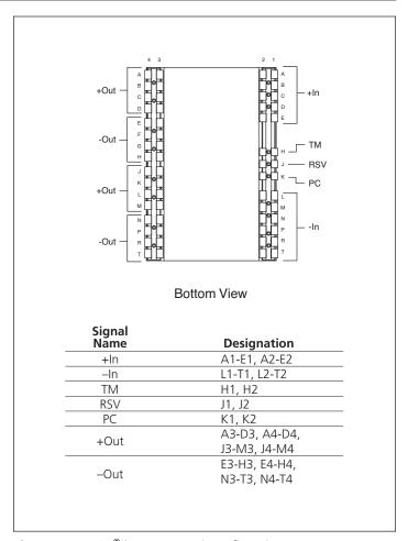
**Figure 14** — BCM<sup>®</sup> bus converter pin configuration
