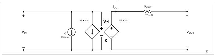
Figure 21 — This model characterizes the DC operation of the bus converter, including the converter transfer function and its losses. The model enables estimates or simulations of output voltage as a function of input voltage and output load, as well as total converter power dissipation or heat generation.
