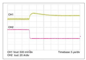
**Figure 11** — 30 – 0 A load step with 100 μF input capacitor and no output capacitor.
