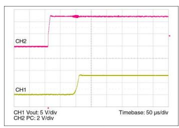
**Figure 2** — Output voltage turn on waveform with PC enabled at full load and  $48 \, V_{\rm IN}$
