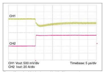
**Figure 10** — 0 – 30 A load step with 100 μF input capacitor and no output capacitor.
