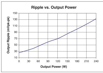
**Figure 9** — Output voltage ripple vs. output power at 48 V<sub>IN</sub> without any external bypass capacitor.
