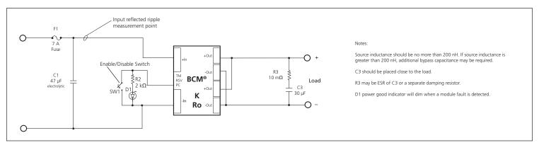
Figure 20 — BCM® module test circuit
