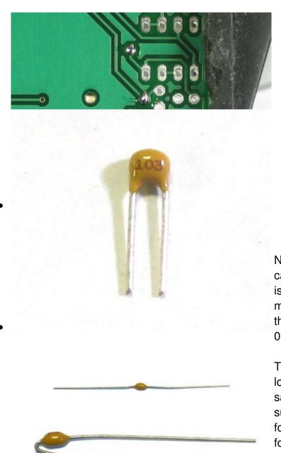
Next is the 0.01uF ceramic capacitor **C8**. The tricky part here is that in older kits there are many 0.1uF ceramic capacitors in the kit that look identical to the 0.01uF!
