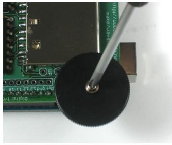
Next you can install the thumbwheel. Use a #0 screwdriver. Align the thumbwheel so it 'grabs' the potentiometer, then gently screw it in place.
