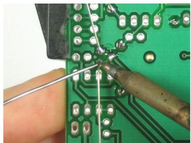
Solder and clip the small capacitor leads.
