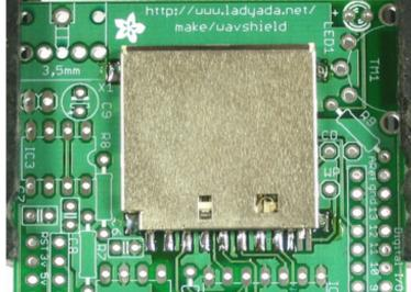
Now go thru and solder the 8 leftmost pins that stick out from the holder. The three rightmost pins are thinner and closer together so they are tougher to solder. Luckily they are not used and you simply skip them (although the photo shows them done).
