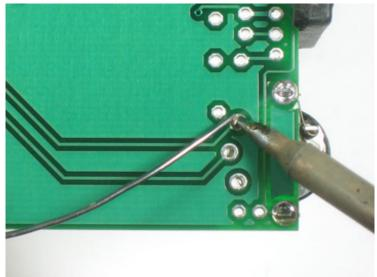
potentiometer. Use plenty of solder so that it has a lot of mechanical strength.
