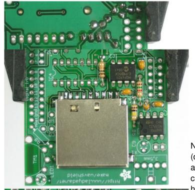
Next is the operational-amplifier (op-amp) **IC3**. It is used to buffer and amplify the output, so that it can drive a small speaker or headphones.
