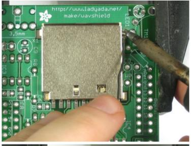
We'll start with the four side tabs that are used to mechanically secure the card holder in place.
