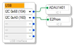
Figure 3. Hardware Configuration Tab
