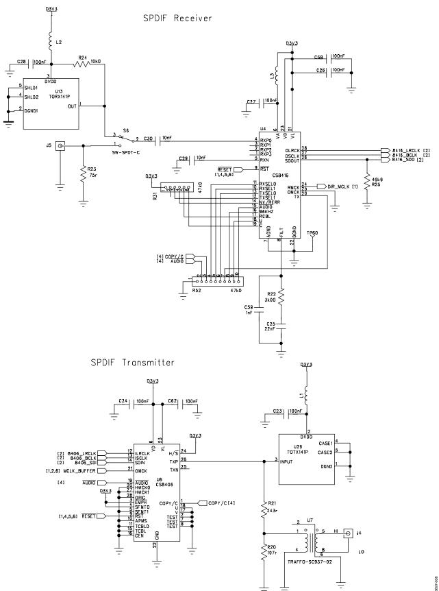
Figure 8. S/PDIF Receiver and Transmitter
