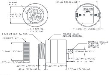
NOTE A: TERMINALS-032 BRASS TIN PLATED, TAPPED FOR #6-32 SCREW. TWO #6-32 NICKEL PLATED BRASS SCREWS INCLUBED. WILL ACCEPT 1/4' OUICK CONNECT.
