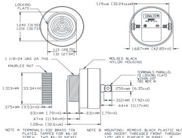
NOTE A: TERMINALS—032 BRASS TIN PLATED, TAPPED FOR #6-32 SCREW. TWO #6-32 NICKEL PLATED BRASS SCREWS INCLUDED. WILL ACCEPT 1/4\* OUICK CONNECT. NOTE B: MOUNTING- REMOVE BLACK PLASTIC NUT
