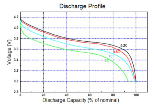
Discharge: 3.0V cutoff at room temperature.
