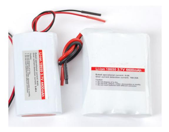
The answer is that these batteries are assembled by a company that is experienced and certified to test and assemble battery packs. The individual batteries are tested and sorted by machine so that each pack has matching batteries with the same capacity and internal resistance. Individuals do not have this equipment, which is why you should not try to make your own packs.
