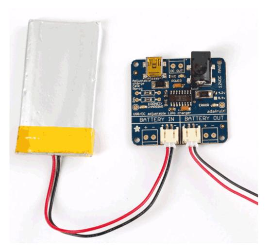
If you want to use the battery while also having it connected to the charger (less plugging and unplugging that way) you can simply use the **BATTERY OUT** connection on the right. The **IN** and **OUT** ports are connected together on the circuit board so it acts as a*pass-through*
