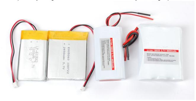
On the left you can see two Lithium Ion Polymer cells. On the right, two packs made of cylindrical Lithium Ion batteries
