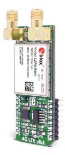
**4G LTE-NA click** carries the LARA-R204 multi-mode cellular module from u-blox. The board is designed to use 5V power supply. I/O voltage levels could be 3.3V or 5V. It communicates with the target microcontroller over UART interface, with additional functionality provided by the following pins on the mikroBUS<sup>TM</sup> line: AN, RST, CS, PWM, INT
