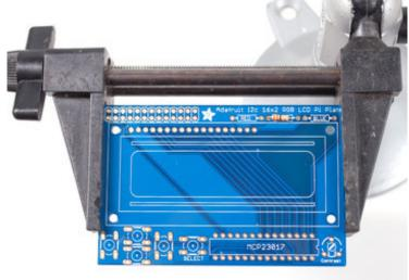
Put the printed circuit board into a vise or board holder, heat up your soldering iron and make sure you're ready to go!
