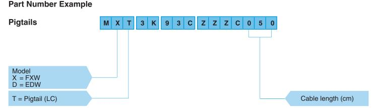
MXT.3K.93C.ZZZC050 = 1 FXW plug (key W), 3K.93C series and one pigtail (LC) on the other side, 50 cm length.
