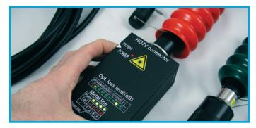
This cable tester provides a quick and easy means of checking the functionality of HD hybrid fibre cables and cable systems. A laser source checks the fibres giving an indication of the attenuation through the whole cable or cable system, and electrical tests check for continuity of both the power and control conductors.
