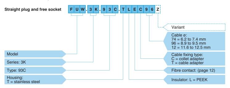
**FUW.3K.93C.TLEC96Z** = Straight plug with keys (W), 3K series, mixed type to accept 2 F2 type fibre optic contacts, 2 power and 2 signal electrical contacts, stainless steel housing, PEEK insulator, female crimp signal contacts, cable fixing type T for 9.2 mm diameter cable, and nut for fitting a bend relief.
