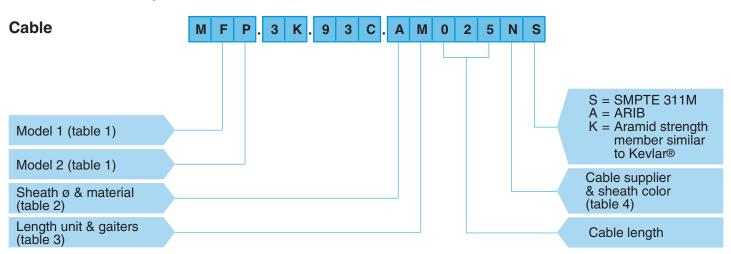
**MFP.3K.93C.AM025NS** = 1 FUW plug and 1 PUW socket (key W), 3K.93C series, on a SMPTE 311M screened cable, 25 m length, sheath ø 9.2 mm, black RAL 9005 jacket color, with GMF/GMP bend relief with cap.
