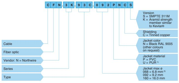
**Note:** 1) PUR outer jacket for high flex and LSZH (Low smoke zero halogen). Recommended for cold temperatures (-40°C). <sup>2)</sup> Recommended for assembly length up to 5 meters.
