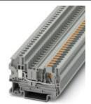
Feed-through terminal block, connection method: Push-in connection, Screw connection, cross section: 0.2 mm² - 6 mm², AWG: 24 - 12, width: 6.2 mm, color: white, mounting: NS 35/7,5, NS 35/15
