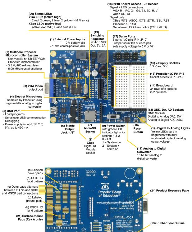
(22) XBee, MicroSD Aux Access (Rev A only)
