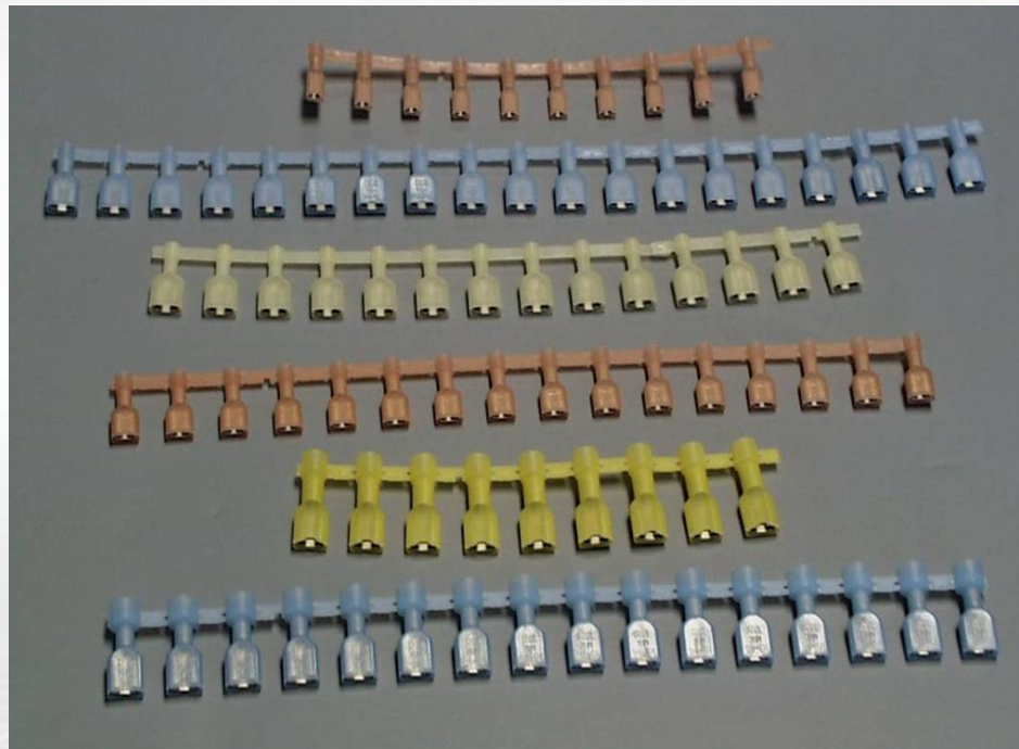
Quixon Fully-Insulated Quick-Disconnect Terminals (Red = 18 to 22 AWG; Blue = 14 to 16 AWG; Yellow = 10 to 12 AWG)
