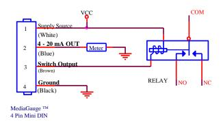
In the example shown above, the MediaGauge MG-MD is attached to an external power supply, a current meter and a relay. We will assume the low set point has been set to 100 psi and the high set point has been set to 375 psi.
