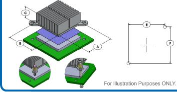
**NOTES:** 1) Dimension A is the length of the heat sink in the direction of the flow.
