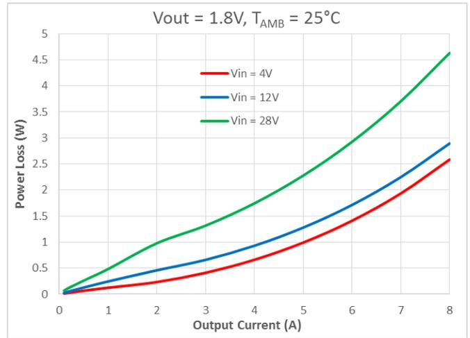
Fig. 8 Power Dissipation vs Output Current (V<sub>OUT</sub>=1.8V)
