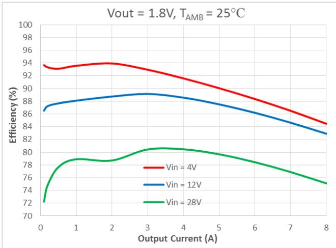
Fig. 7 Efficiency vs Output Current (V<sub>OUT</sub>=1.8V)
