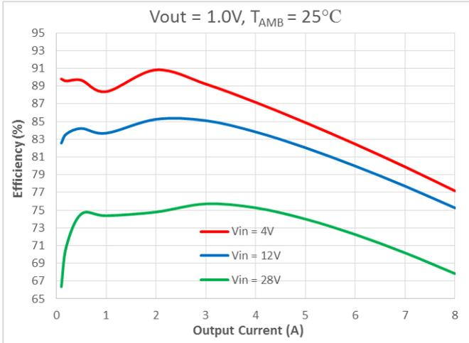
Fig. 9 Efficiency vs Output Current (V<sub>OUT</sub>=1.0V)
