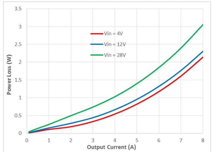
Fig. 12 Power Dissipation vs Output Current (V<sub>OUT</sub>=0.6V)
