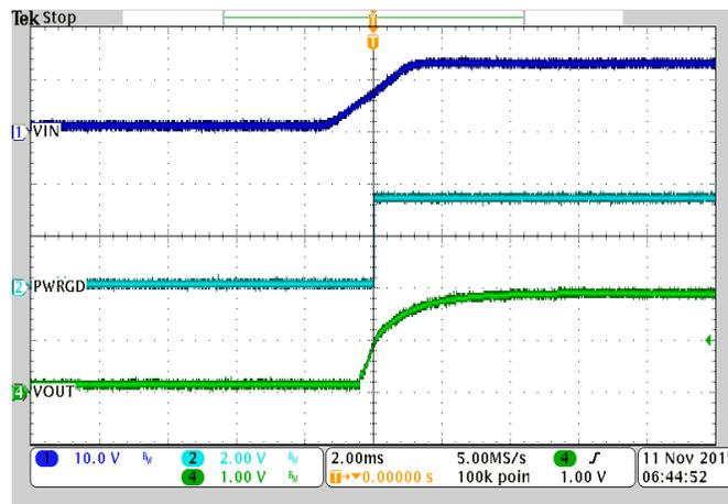
Fig. 17 Start-Up Waveforms for SPM1006
