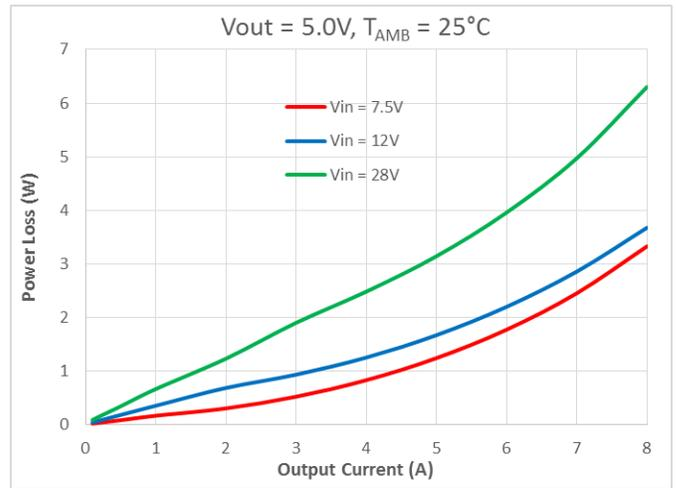
Fig. 4 Power Dissipation vs Output Current (V<sub>OUT</sub>=5V)
