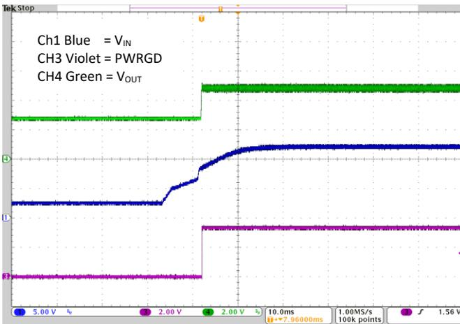
Fig. 20 Start-up with pre-bias 2.62V ( $V_{OUT}=5V$ )
