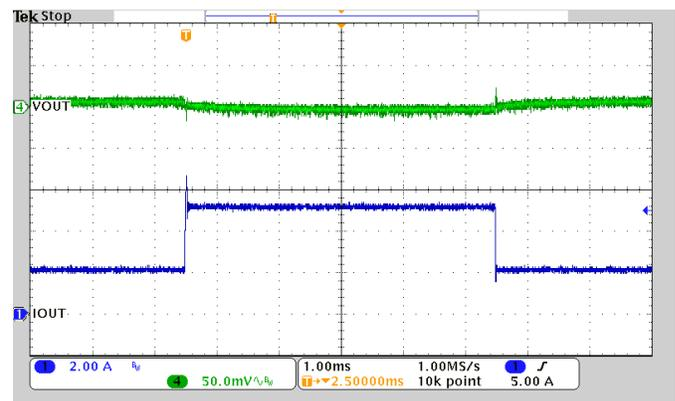
Fig. 26 Transient Response (V<sub>IN</sub> = 12V, V<sub>OUT</sub> = 0.6V)
