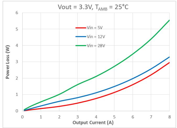
Fig. 6 Power Dissipation vs Output Current (V<sub>OUT</sub>=3.3V)
