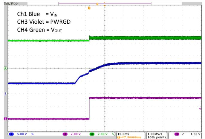
Fig. 21 Start-up with pre-bias 4.21V ( $V_{OUT}=5V$ )
