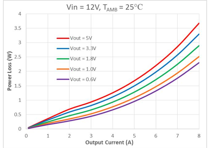
Fig. 2 Power Dissipation vs Output Current (V<sub>IN</sub>=12V)
