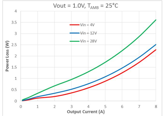
Fig. 10 Power Dissipation vs Output Current (V<sub>OUT</sub>=1.0V)
