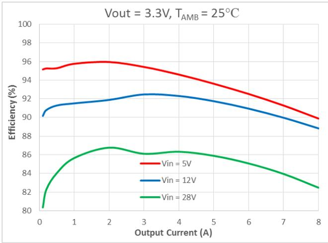
Fig. 5 Efficiency vs Output Current (V<sub>OUT</sub>=3.3V)
