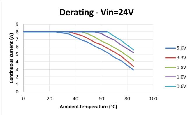
Fig. 31 Output current derating (24V input)
