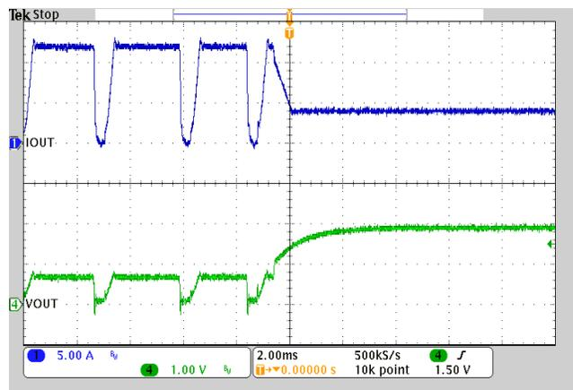
Fig. 28 Recovery from overcurrent
