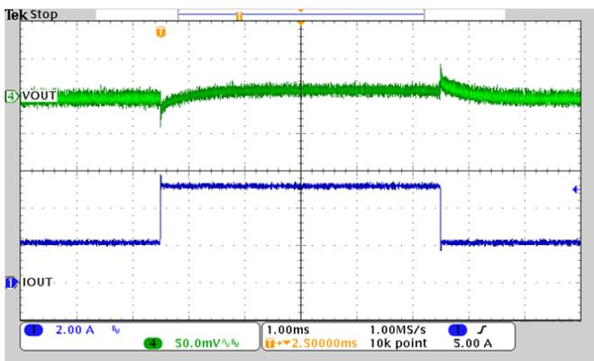
Fig. 25 Transient Response (V<sub>IN</sub> = 12V, V<sub>OUT</sub> = 5V)
