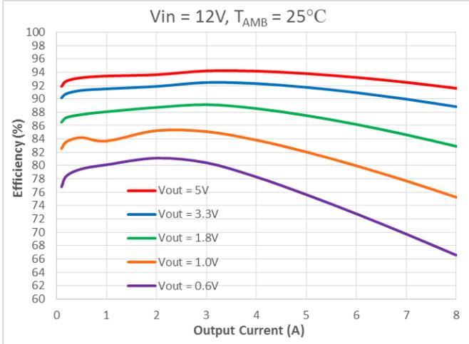
Fig. 1 Efficiency vs Output Current (V<sub>IN</sub>=12V)
