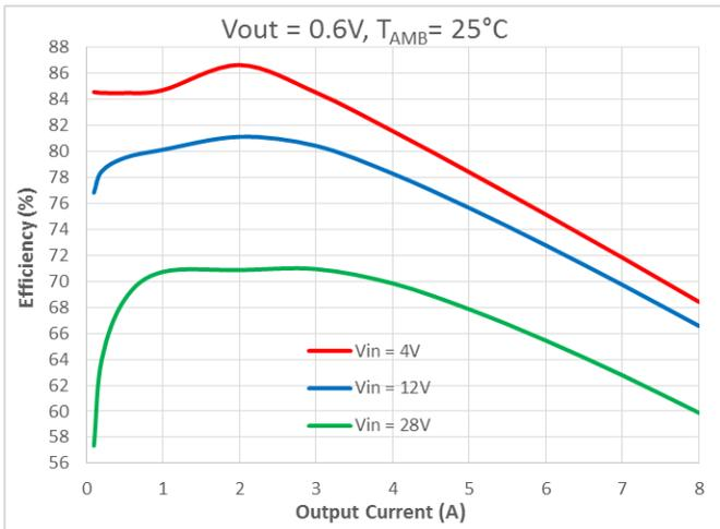
Fig. 11 Efficiency vs Output Current (V<sub>OUT</sub>=0.6V)
