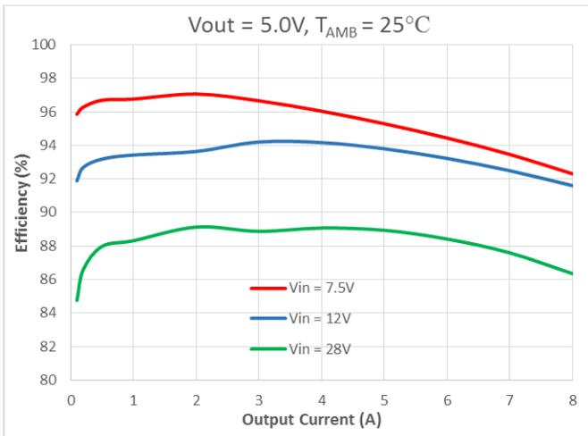
Fig. 3 Efficiency vs Output Current (V<sub>OUT</sub>=5V)
