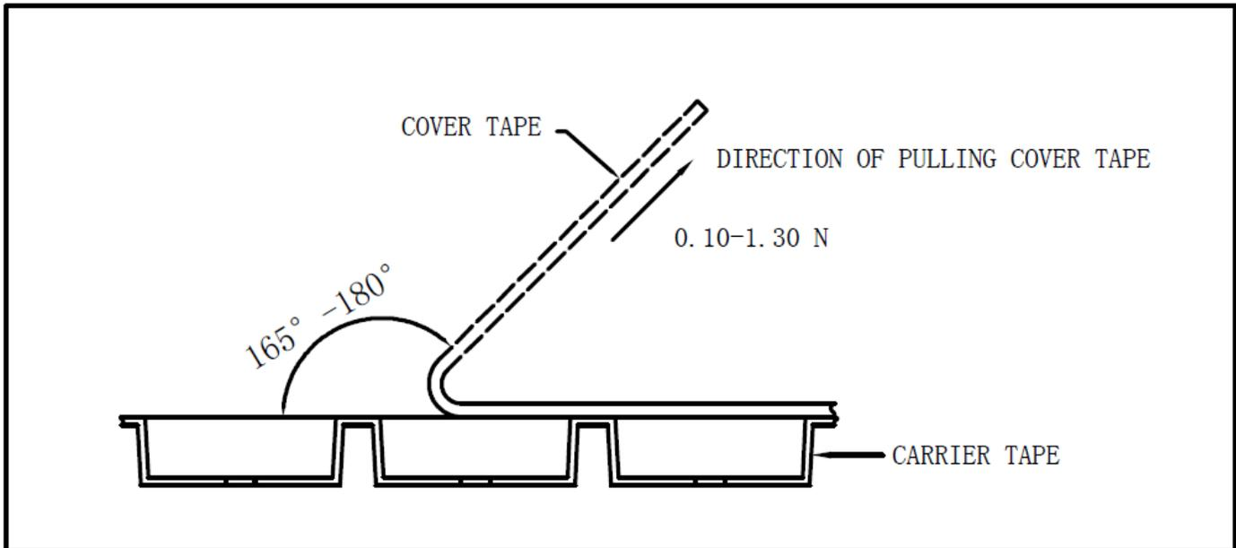
Fig. 35 Peel Speed and Strength of Cover Tape
