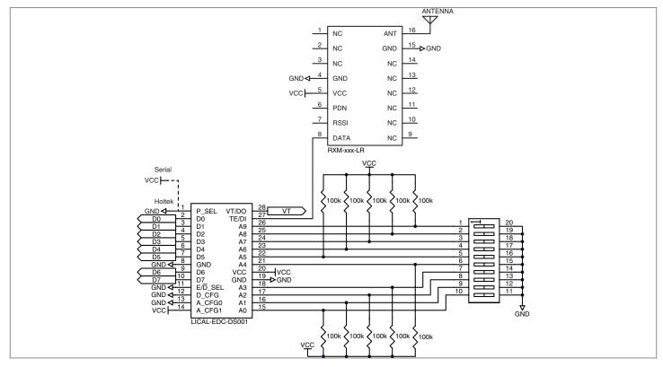
LR Receiver and DS Decoder Schematic
