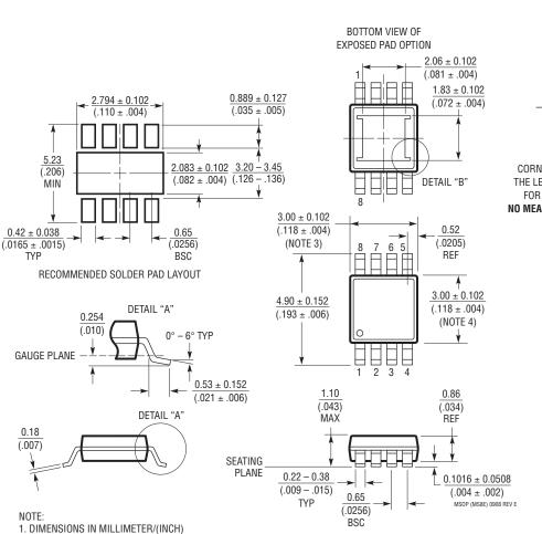
MS8E Package 8-Lead Plastic MSOP, Exposed Die Pad (Reference LTC DWG # 05-08-1662 Rev E)
