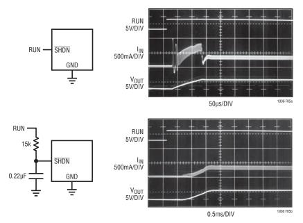
Figure 5. To Soft-Start the LT1936, Add a Resistor and Capacitor to the SHDN Pin.  $V_{IN}$  = 12V,  $V_{OUT}$  = 3.3V,  $C_{OUT}$  = 2  $\times$  22µF,  $R_{LOAD}$  = 3.3 $\Omega$
