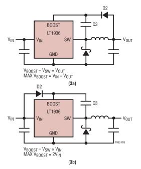
Figure 3. Two Circuits for Generating the Boost Voltage
