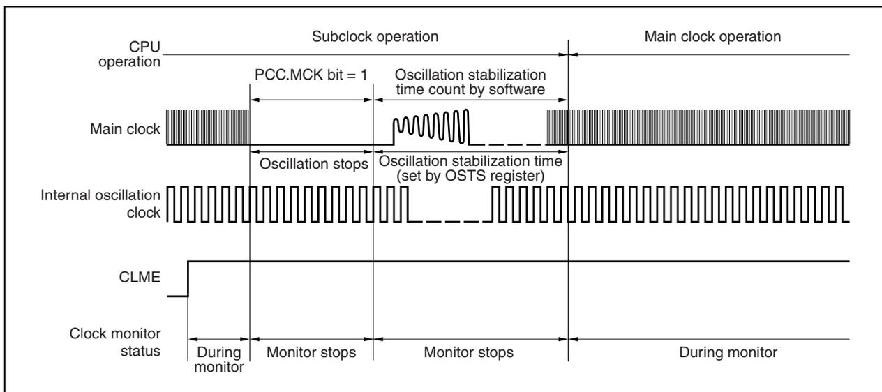
**(5) Operation while CPU is operating on internal oscillation clock (CCLS.CCLS bit = 1)**
