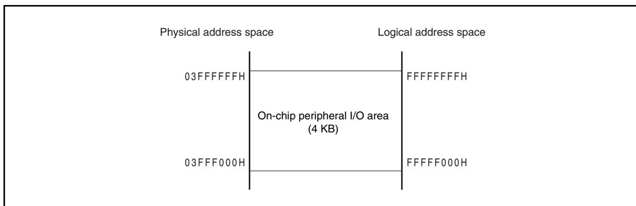
Peripheral I/O registers that have functions to specify the operation mode for and monitor the status of the on-chip peripheral I/O are mapped to the on-chip peripheral I/O area. Program cannot be fetched from this area.
