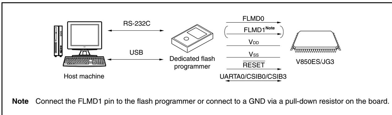
A host machine is required for controlling the dedicated flash programmer.
