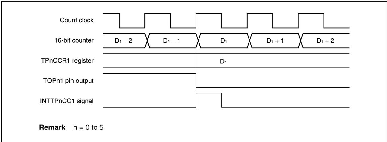
Usually, the INTTPnCC1 signal is generated when the 16-bit counter counts up next time after its count value matches the value of the TPnCCR1 register.
