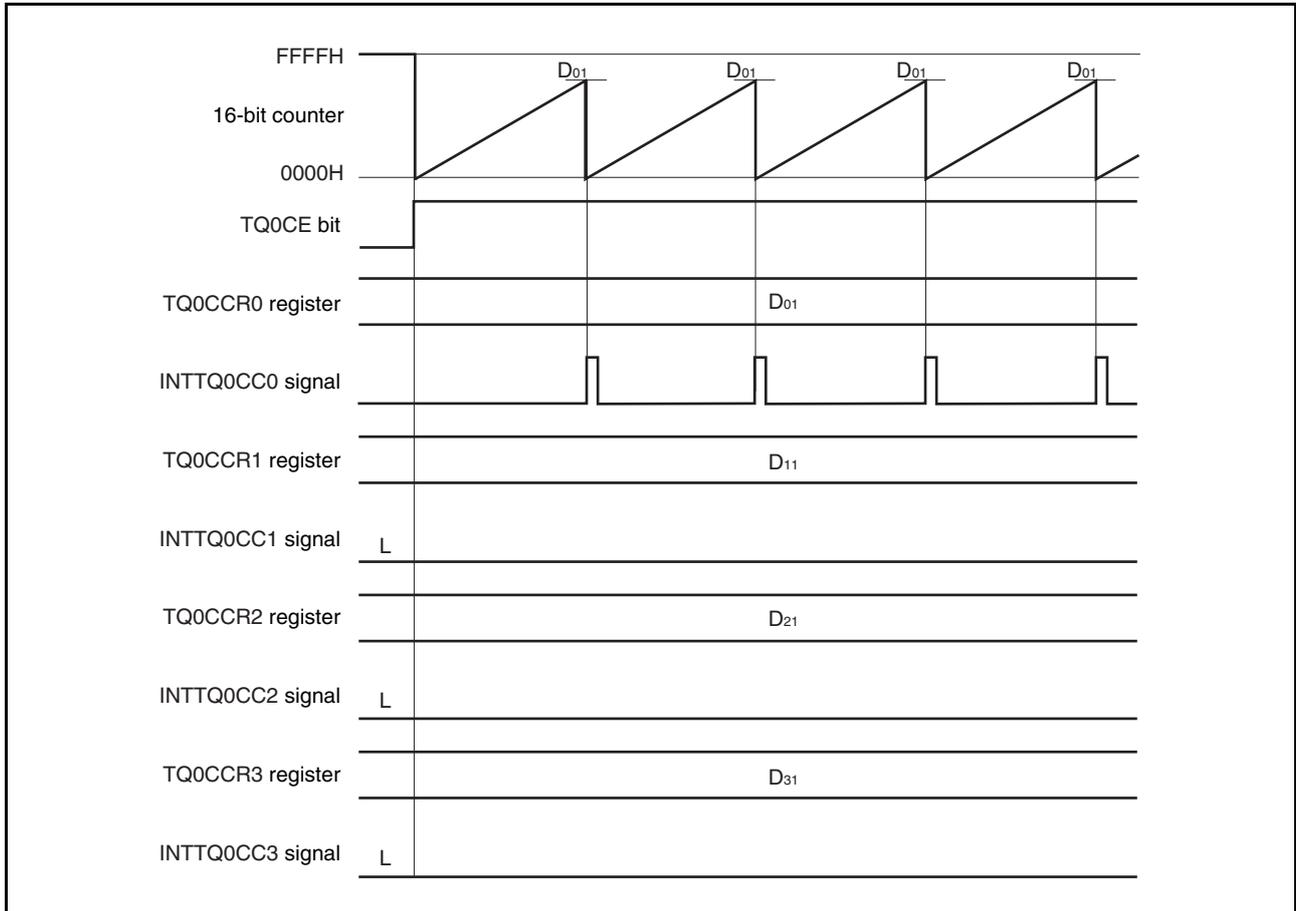
**8.5.3 External trigger pulse output mode (TQ0MD2 to TQ0MD0 bits = 010)**
