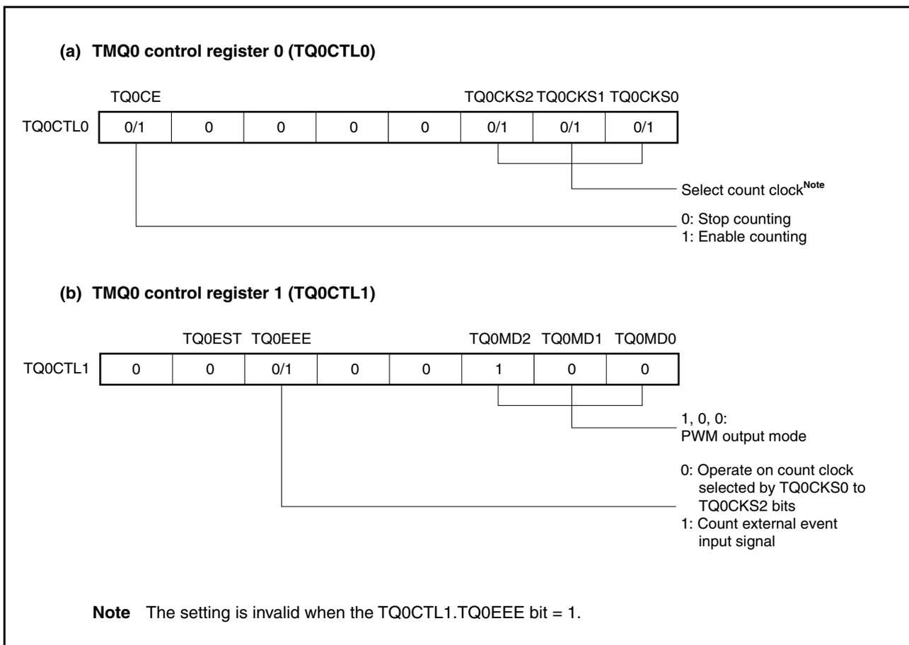
Figure 8-26. Register Setting for Operation in PWM Output Mode (2/3)
