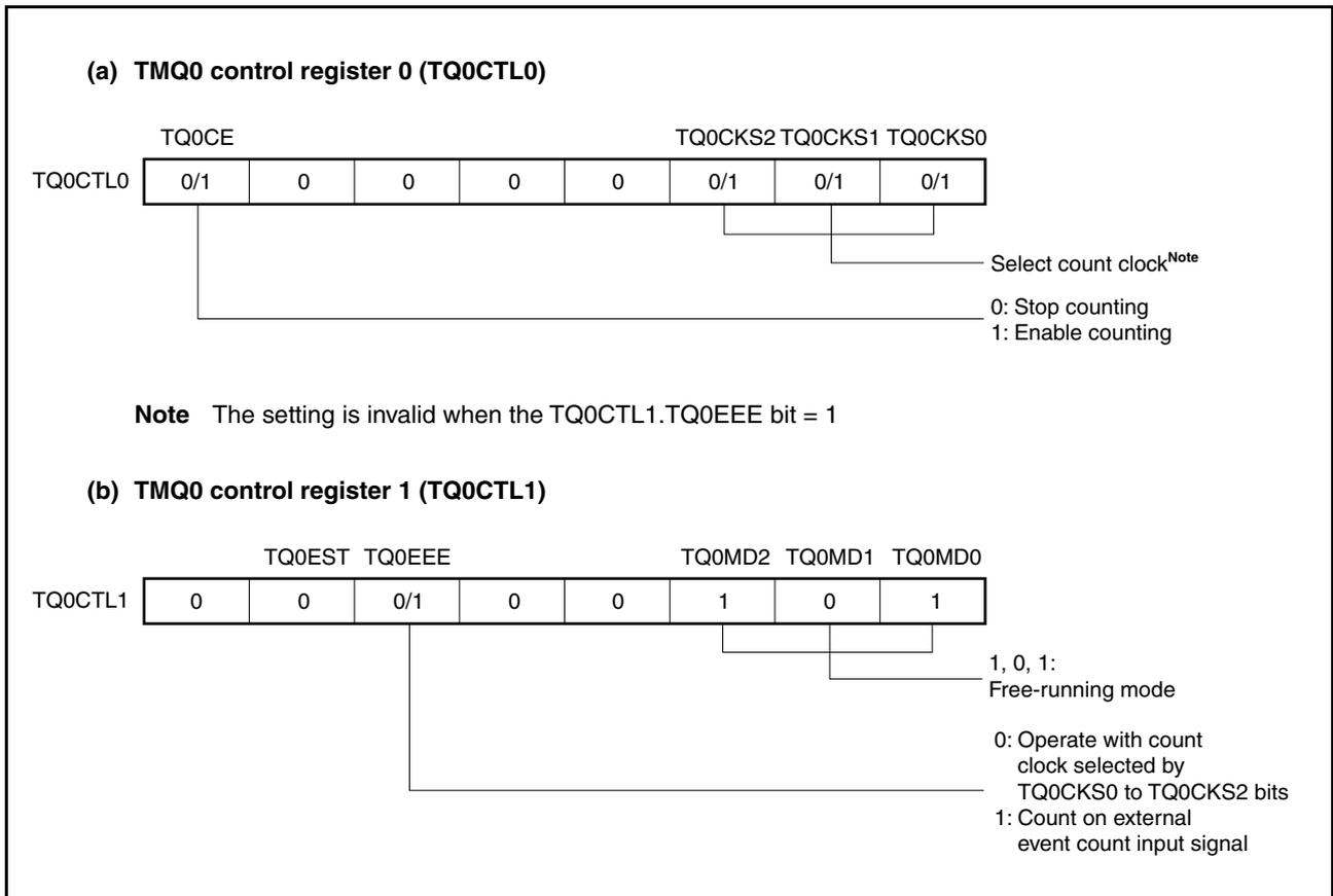
Figure 8-31. Register Setting in Free-Running Timer Mode (2/3)
