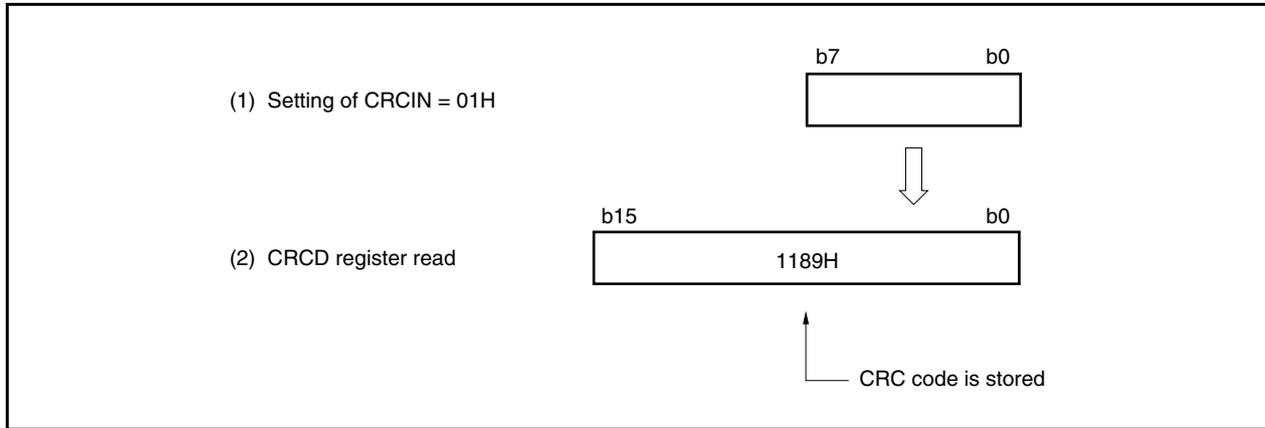
The code when 01H is sent LSB first is (1000 0000). Therefore, the CRC code from generation polynomial  $X^{16} + X^{12} + X^5 + 1$  becomes the remainder when  $(1000\ 0000) X^{16}$  is divided by  $(1\ 0001\ 0000\ 0010\ 0001)$  using the modulo-2 operation formula.
