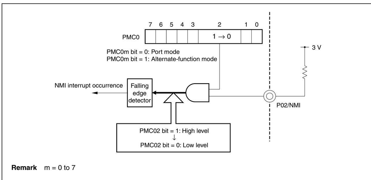
(2) In port mode, the PF<sub>n</sub>.PF<sub>nm</sub> bit is valid only in the output mode (PM<sub>n</sub>.PM<sub>nm</sub> bit = 0). In the input mode (PM<sub>nm</sub> bit = 1), the value of the PF<sub>nm</sub> bit is not reflected in the buffer.
