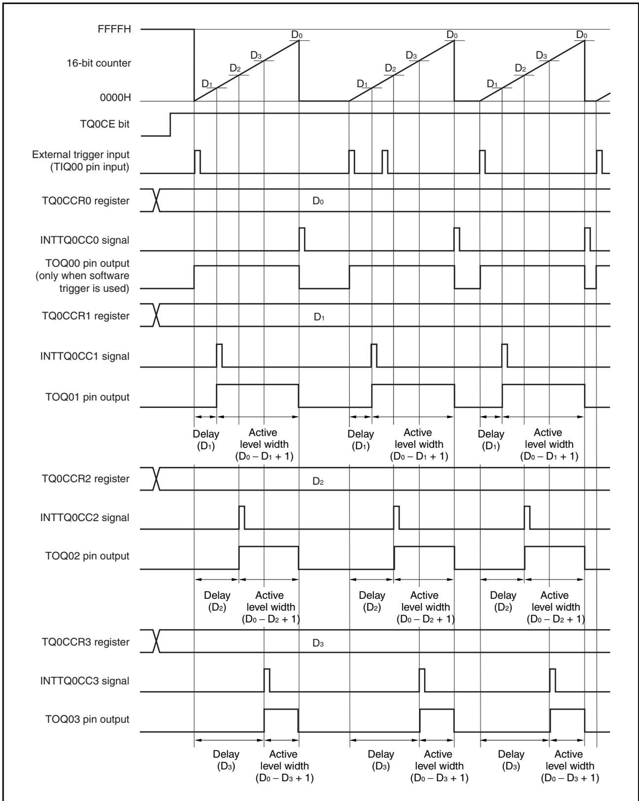
When the TQ0CE bit is set to 1, 16-bit timer/event counter Q waits for a trigger. When the trigger is generated, the 16-bit counter is cleared from FFFFH to 0000H, starts counting, and outputs a one-shot pulse from the TOQ0k pin. After the one-shot pulse is output, the 16-bit counter is set to FFFFH, stops counting, and waits for a trigger. If a trigger is generated again while the one-shot pulse is being output, it is ignored.
