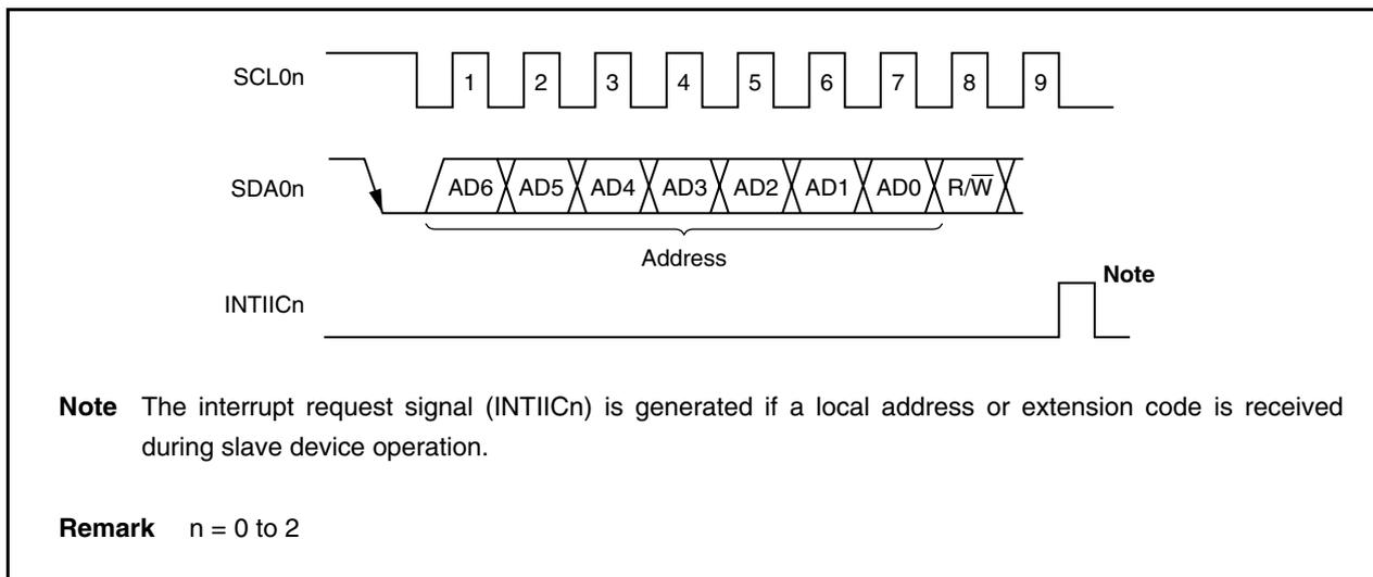
The slave address and the eighth bit, which specifies the transfer direction as described in **17.6.3 Transfer direction specification** below, are written together to IIC shift register  $n$  (IICn) and then output. Received addresses are written to the IICn register ( $n = 0$  to 2).
