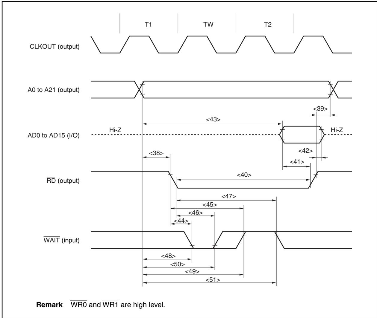
**(b) Write cycle (CLKOUT asynchronous): In separate bus mode****( $T_A = -40$  to  $+85^\circ\text{C}$ ,  $V_{DD} = EV_{DD} = AV_{REF0} = AV_{REF1}$ ,  $V_{SS} = EV_{SS} = AV_{SS} = 0$  V,  $C_L = 50$  pF)**
