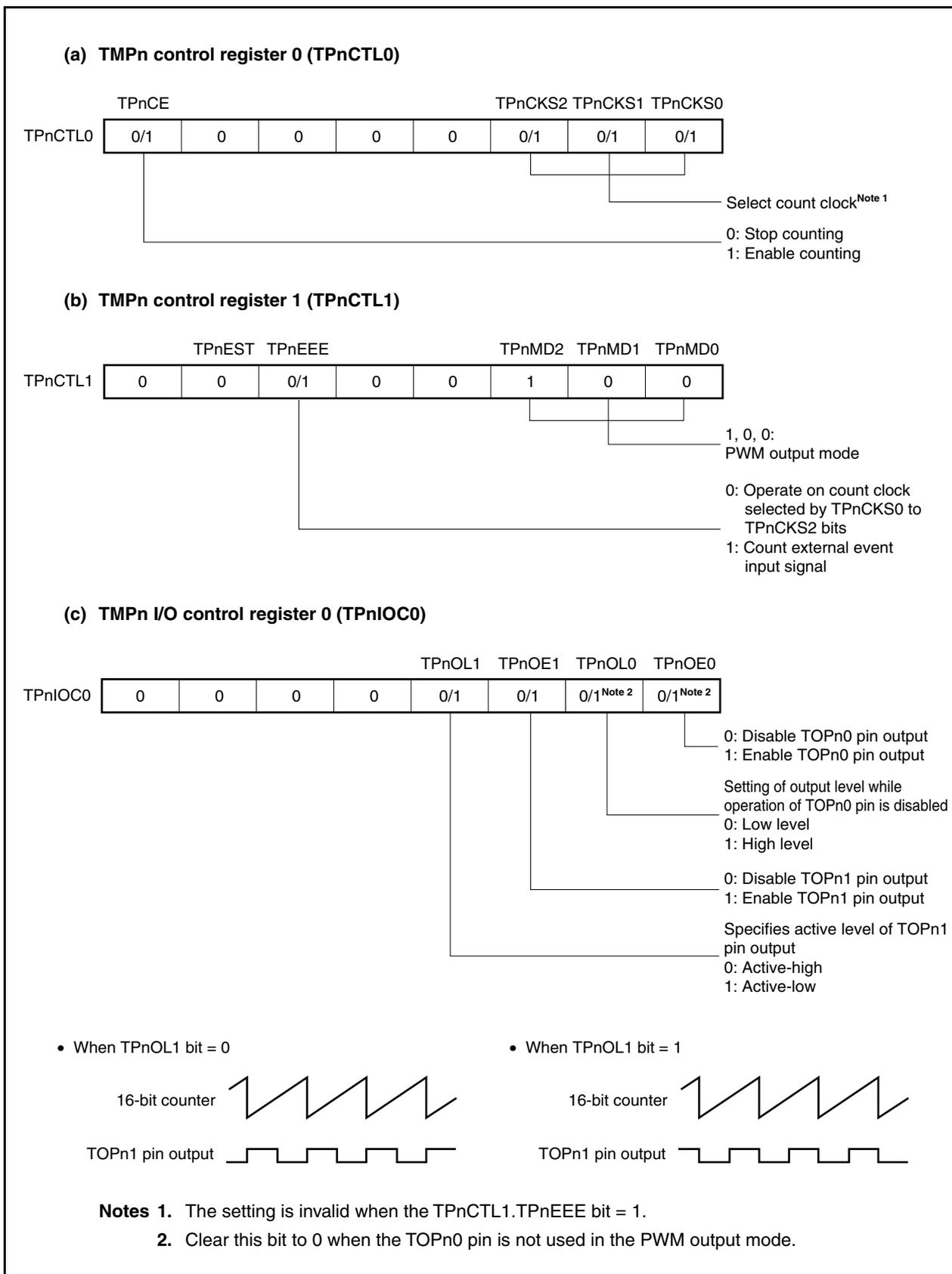
Figure 7-26. Register Setting for Operation in PWM Output Mode (2/2)
