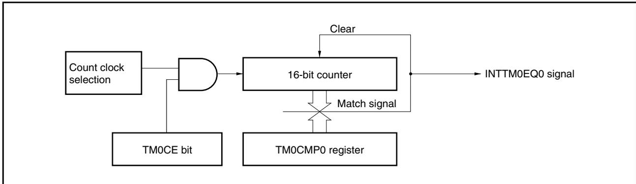
Figure 9-3. Basic Timing of Operation in Interval Timer Mode
