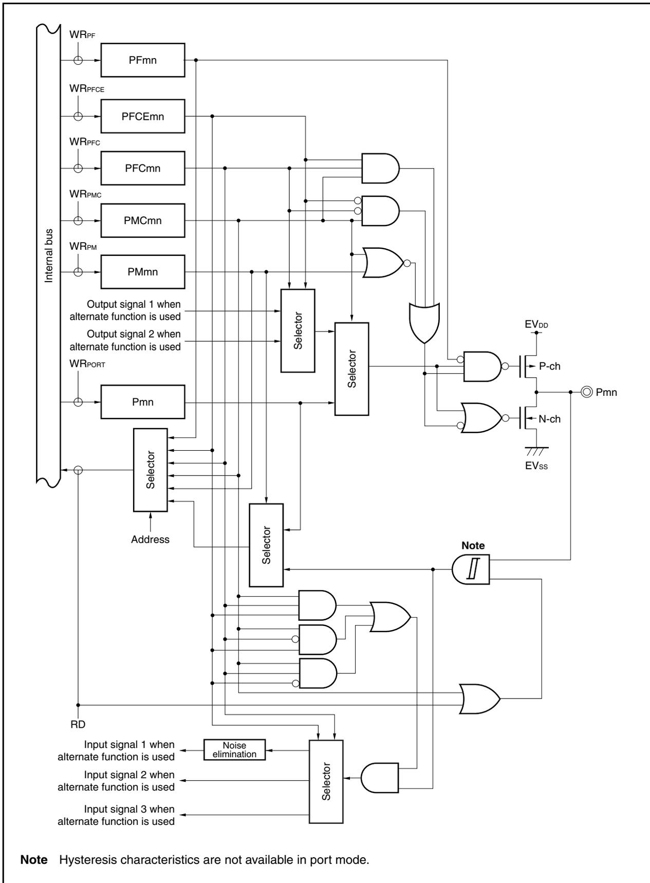
Figure 4-28. Block Diagram of Type U-12
