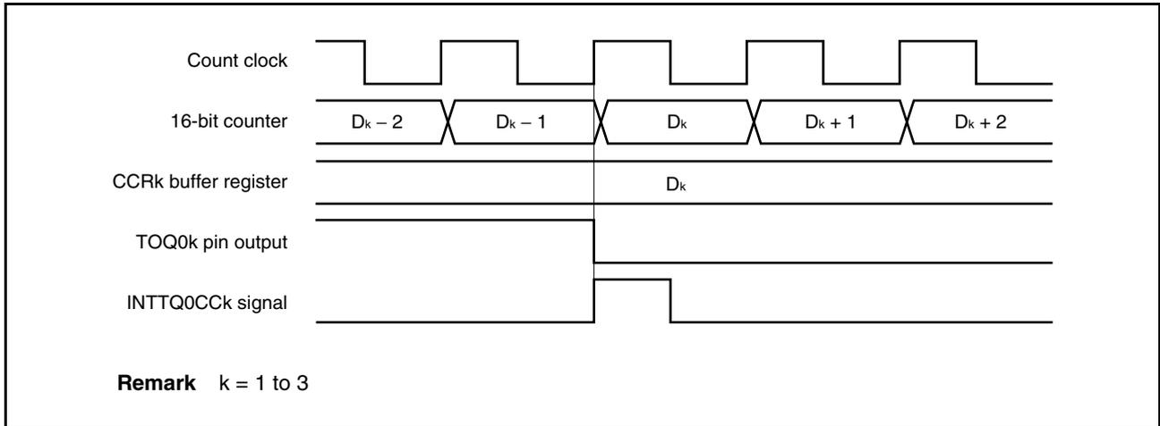
Usually, the INTTQ0CCK signal is generated in synchronization with the next counting up after the count value of the 16-bit counter matches the value of the TQ0CCRk register.
