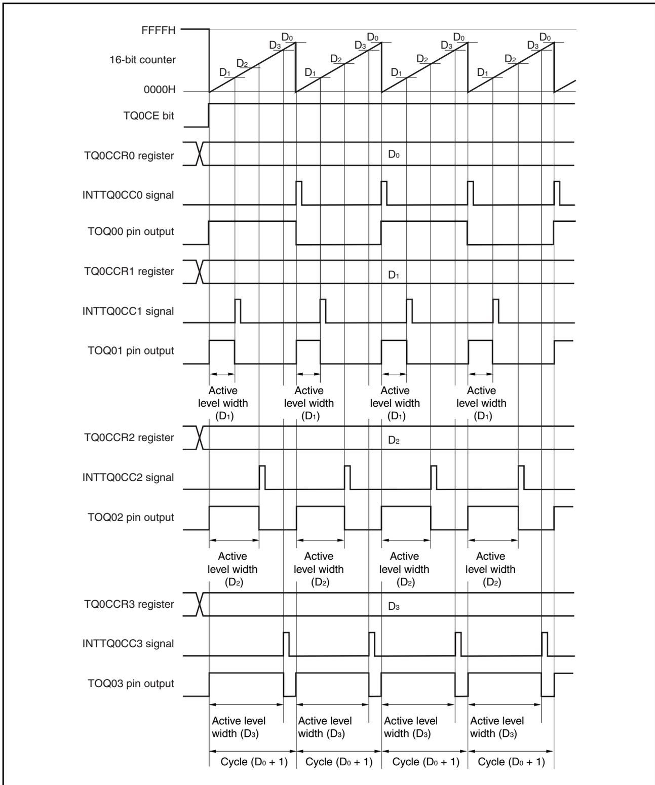
When the TQ0CE bit is set to 1, the 16-bit counter is cleared from FFFFH to 0000H, starts counting, and outputs PWM waveform from the TQ0k pin.
