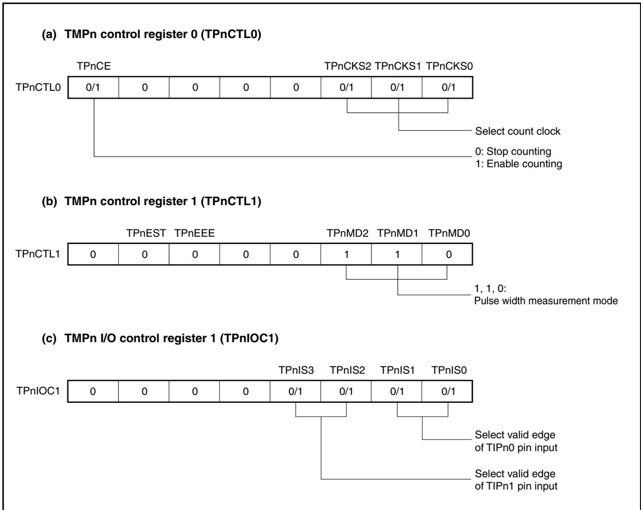
Figure 7-36. Register Setting in Pulse Width Measurement Mode (2/2)
