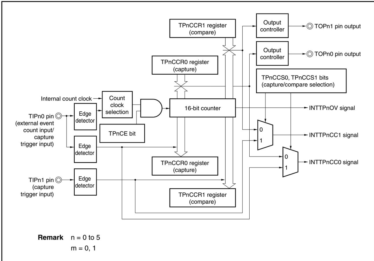
When the TPnCE bit is set to 1, 16-bit timer/event counter P starts counting, and the output signals of the TOPn0 and TOPn1 pins are inverted. When the count value of the 16-bit counter later matches the set value of the TPnCCRm register, a compare match interrupt request signal (INTTPnCCm) is generated, and the output signal of the TOPnm pin is inverted.
