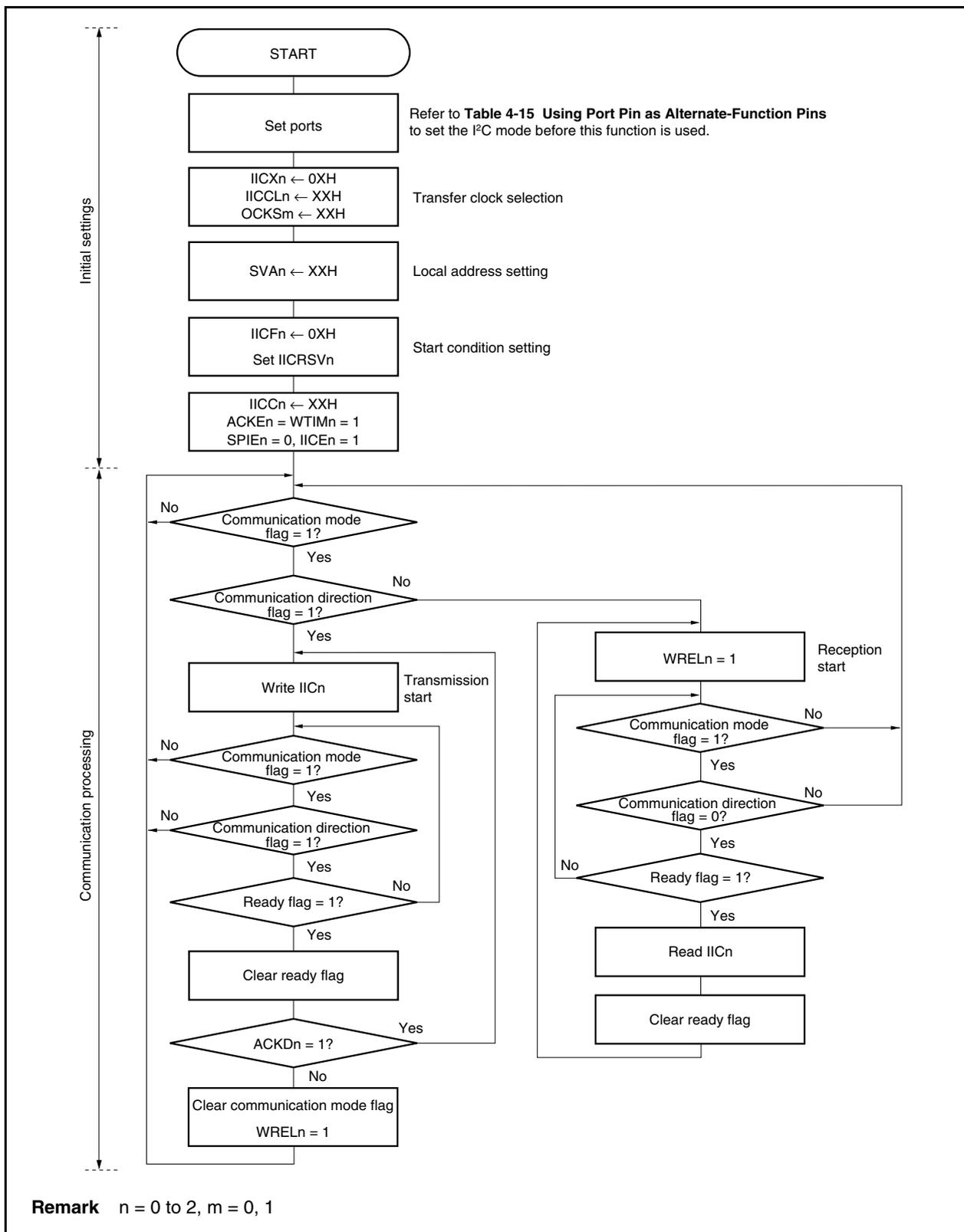
The following shows an example of the processing of the slave device by an INTIICn interrupt (it is assumed that no extension codes are used here). During an INTIICn interrupt, the status is confirmed and the following steps are executed.
