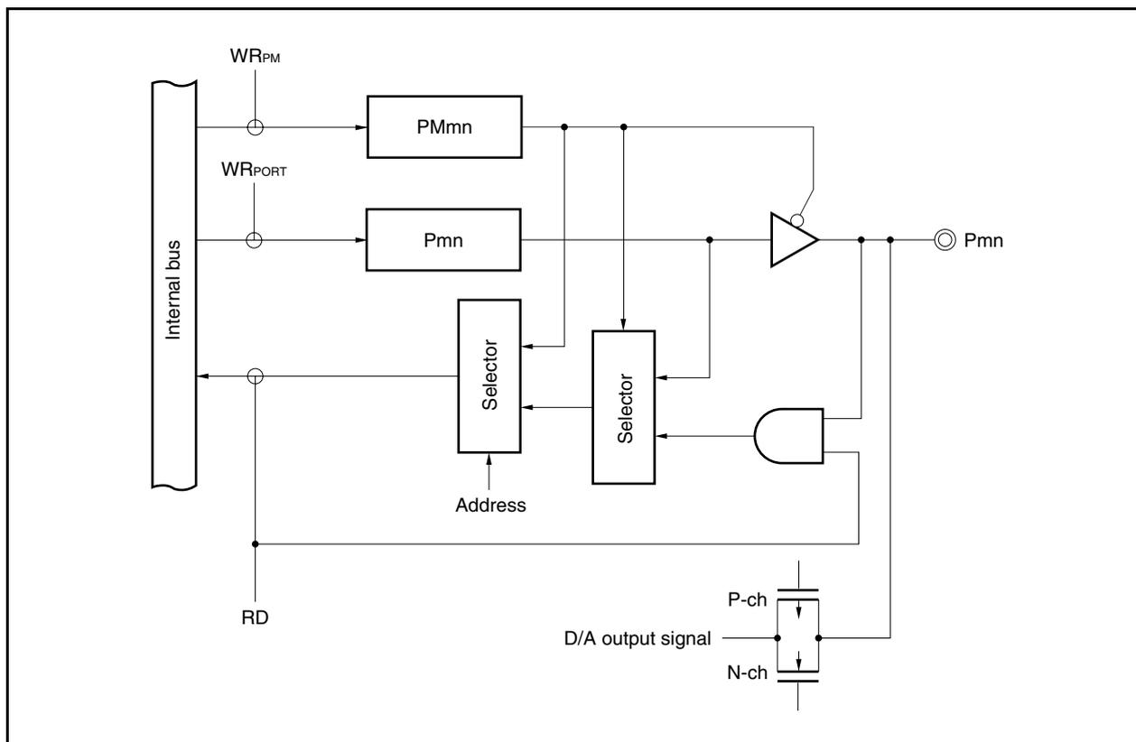
Figure 4-5. Block Diagram of Type C-1
