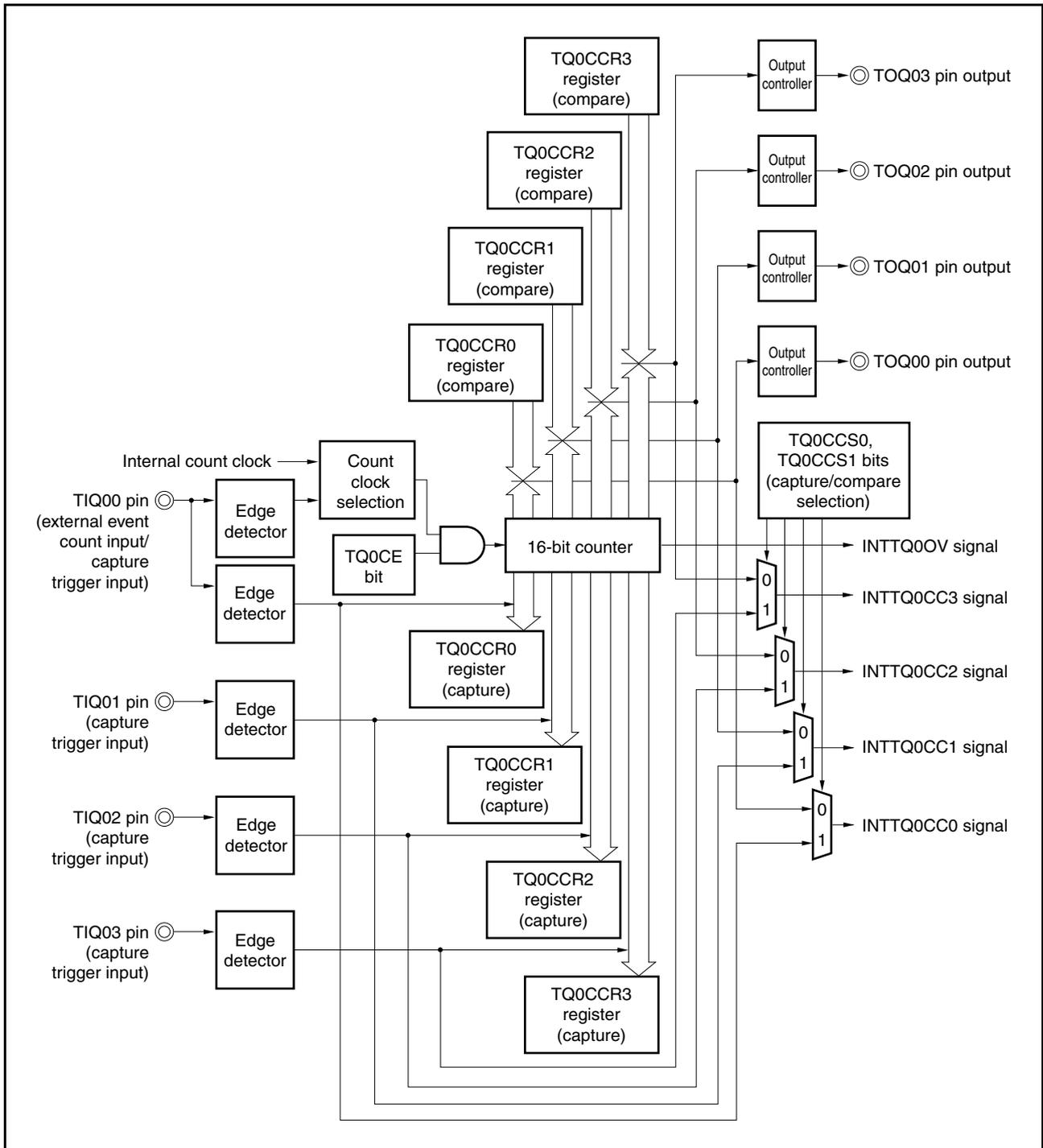
When the TQ0CE bit is set to 1, 16-bit timer/event counter Q starts counting, and the output signals of the TOQ00 to TOQ03 pins are inverted. When the count value of the 16-bit counter later matches the set value of the TQ0CCRm register, a compare match interrupt request signal (INTTQ0CCm) is generated, and the output signal of the TOQ0m pin is inverted.
