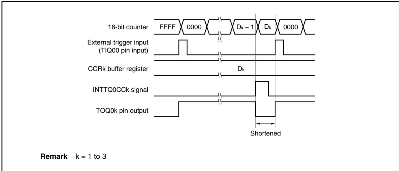
If the trigger is detected immediately before the INTTQ0CCk signal is generated, the INTTQ0CCk signal is not generated, and the 16-bit counter is cleared to 0000H and continues counting. The output signal of the TOQ0k pin remains active. Consequently, the active period of the PWM waveform is extended.
