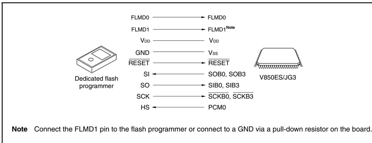
The dedicated flash programmer outputs the transfer clock, and the V850ES/JG3 operates as a slave.
