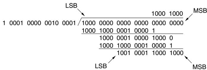
Therefore, the CRC code becomes  $\overbrace{1001}^9 \overbrace{0001}^8 \overbrace{1000}^1 \overbrace{1000}^1$ . Since LSB first is used, this corresponds to 1189H in hexadecimal notation.
