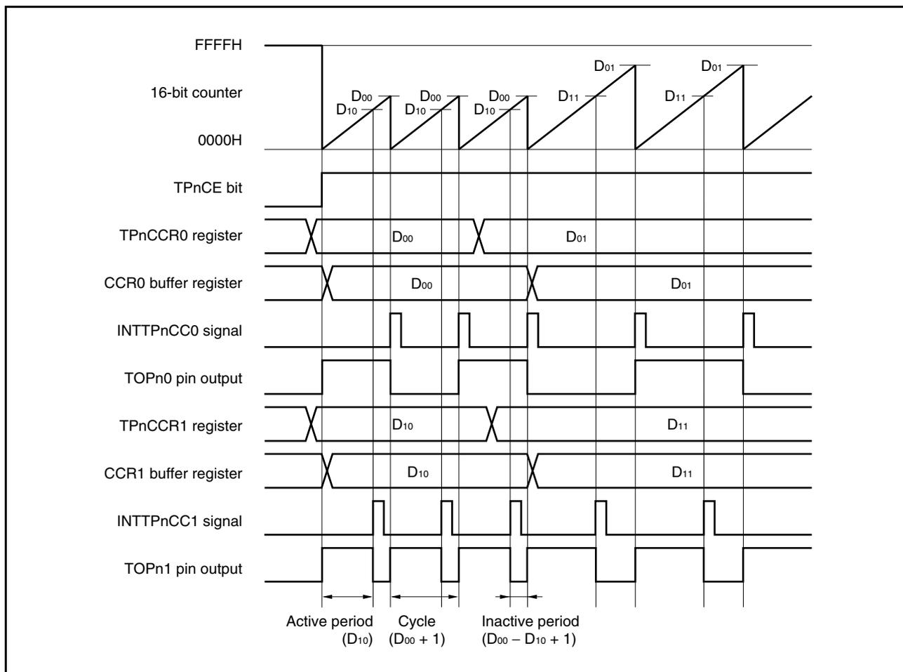
When the TPnCE bit is set to 1, the 16-bit counter is cleared from FFFFH to 0000H, starts counting, and outputs a PWM waveform from the TOPn1 pin.
