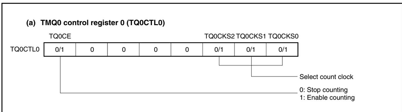
Figure 8-18. Register Setting for Operation in External Trigger Pulse Output Mode (2/3)
