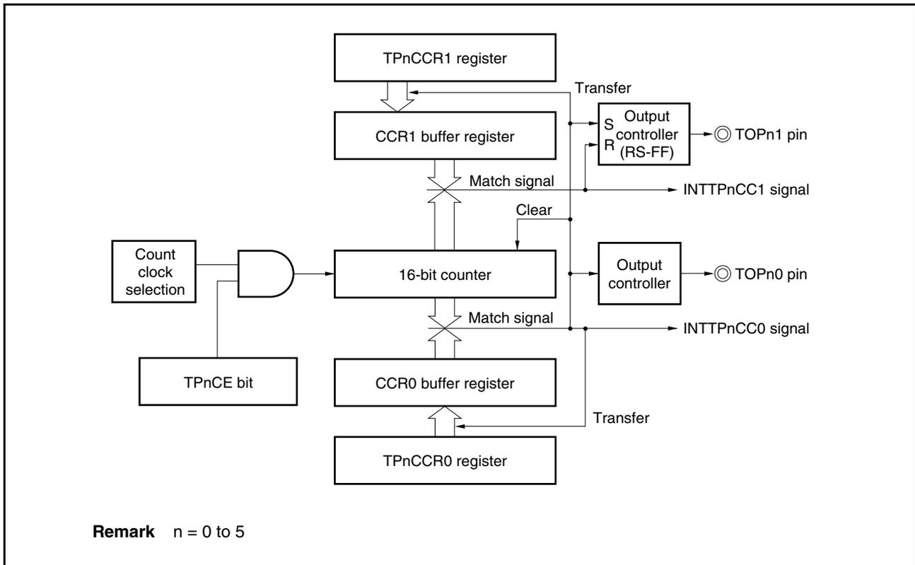
Figure 7-25. Basic Timing in PWM Output Mode
