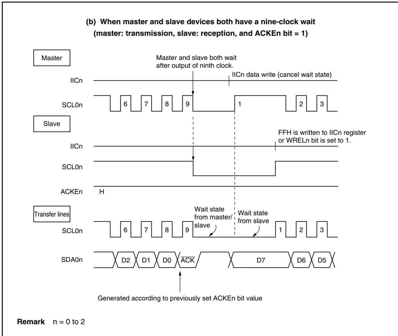
A wait state may be automatically generated depending on the setting of the IICn.WTIMn bit (n = 0 to 2).
