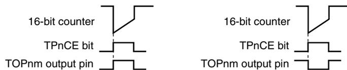
**Cautions** 1. Rewrite the TPnOL1, TPnOE1, TPnOL0, and TPnOE0 bits when the TPnCTL0.TPnCE bit = 0. (The same value can be written when the TPnCE bit = 1.) If rewriting was mistakenly performed, clear the TPnCE bit to 0 and then set the bits again.
