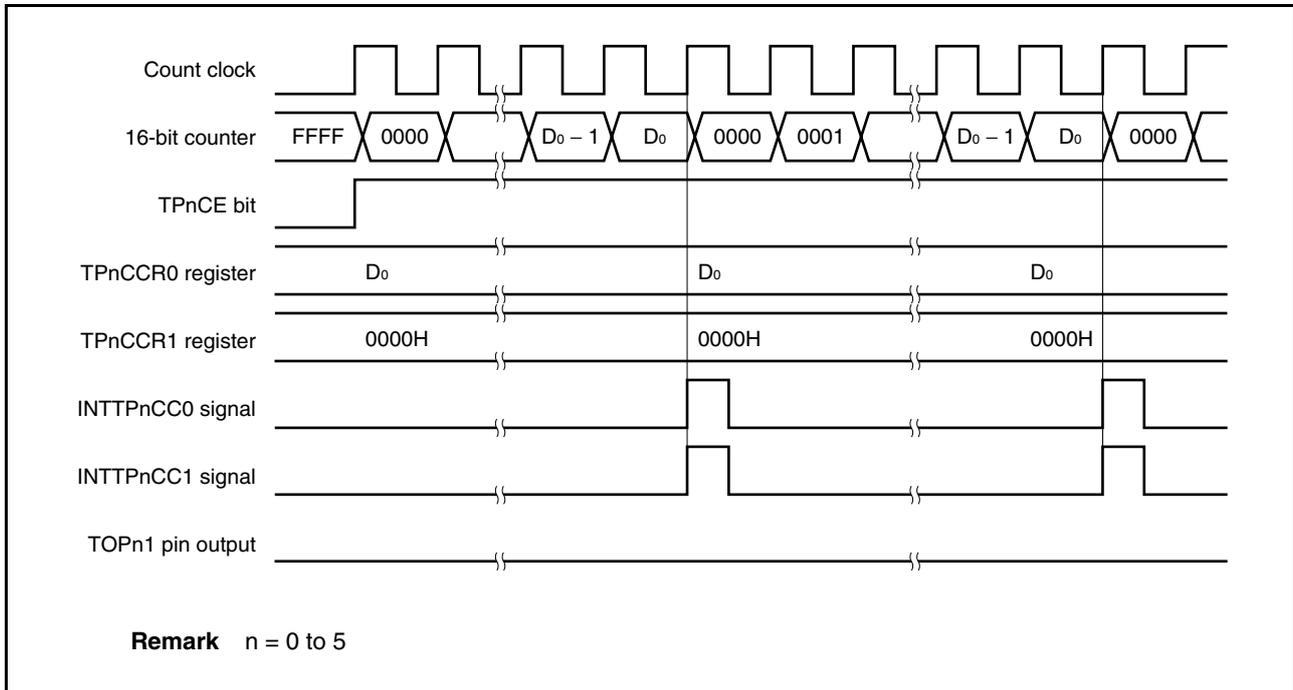
To output a 100% waveform, set a value of (set value of TPnCCR0 register + 1) to the TPnCCR1 register. If the set value of the TPnCCR0 register is FFFFH, 100% output cannot be produced.
