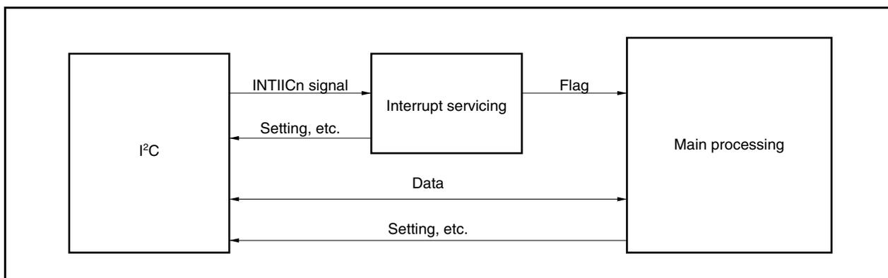
Therefore, the following three flags are prepared so that the data transfer processing can be performed by transmitting these flags to the main processing instead of INTIICn signal.
