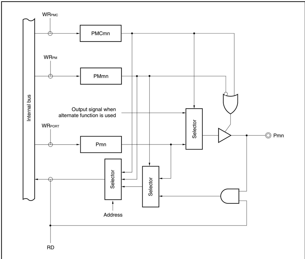
Figure 4-8. Block Diagram of Type D-3
