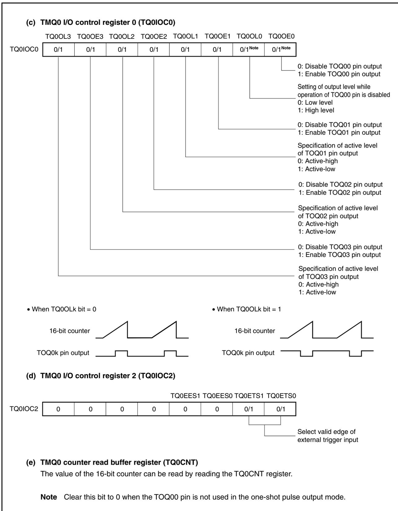
Figure 8-22. Register Setting for Operation in One-Shot Pulse Output Mode (3/3)
