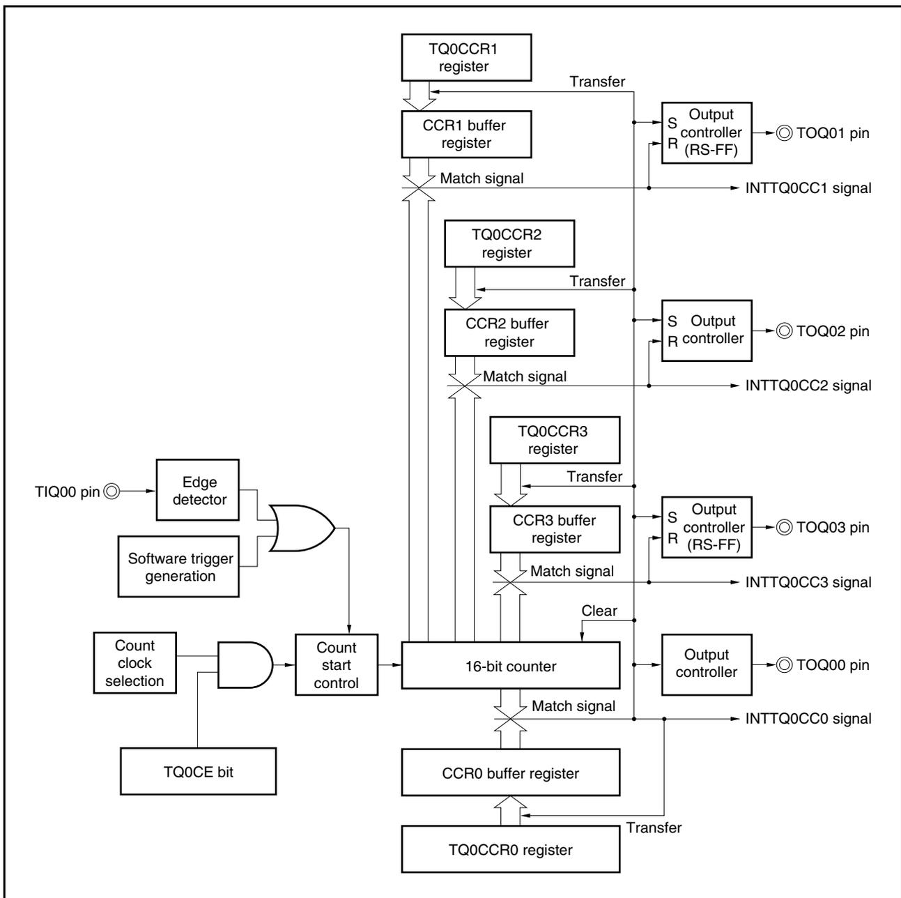
pin. If the trigger is generated again while the counter is operating, the counter is cleared to 0000H and restarted. (The output of the TOQ00 pin is inverted. The TOQ0k pin outputs a high-level regardless of the status (high/low) when a trigger is generated.)
