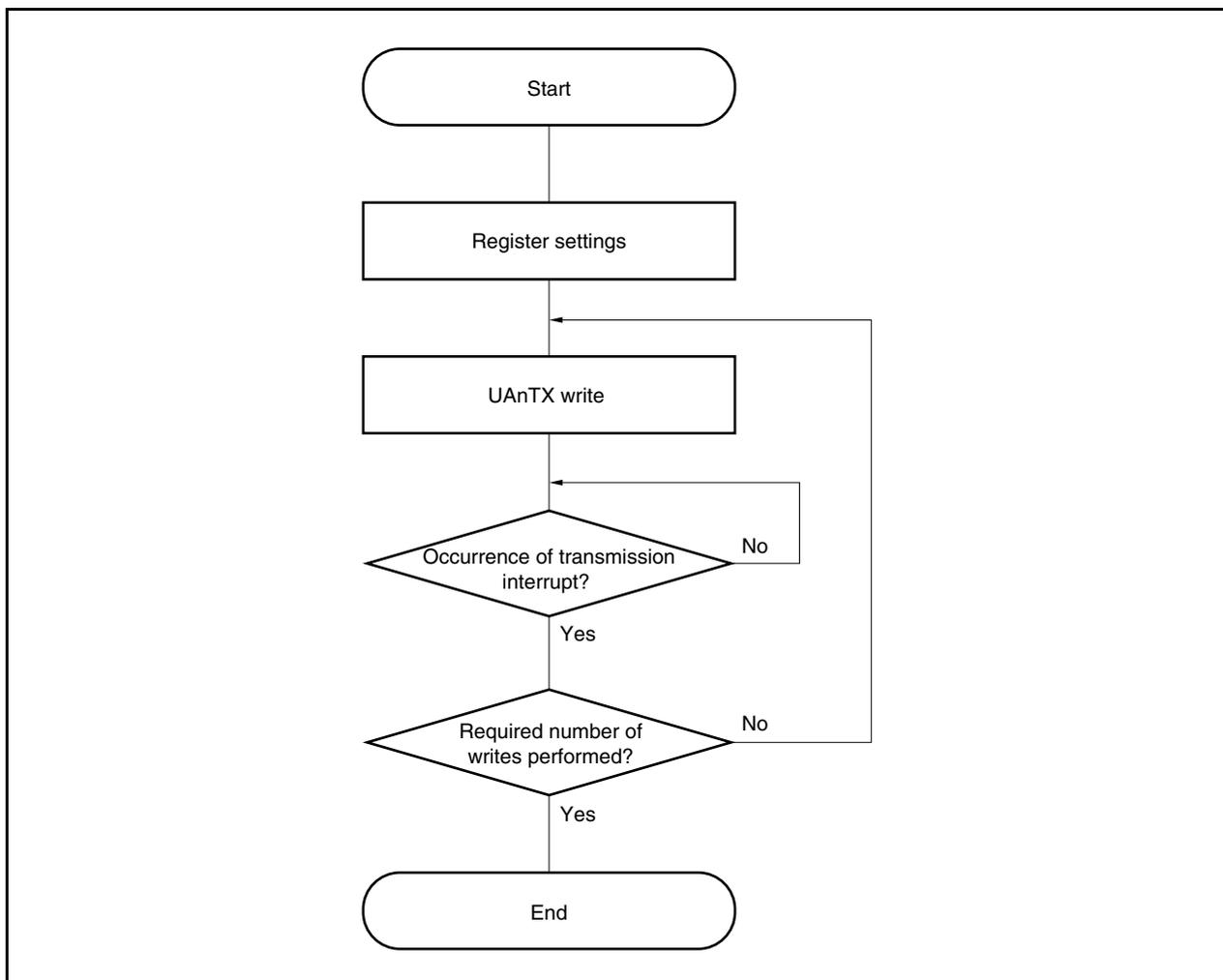
Figure 15-12. Continuous Transmission Operation Timing
