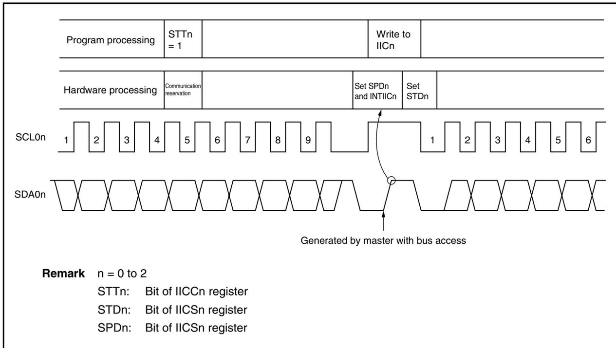
Communication reservations are accepted via the following timing. After the IICSn.STDn bit is set to 1, a communication reservation can be made by setting the IICn.STTn bit to 1 before a stop condition is detected (n = 0 to 2).
