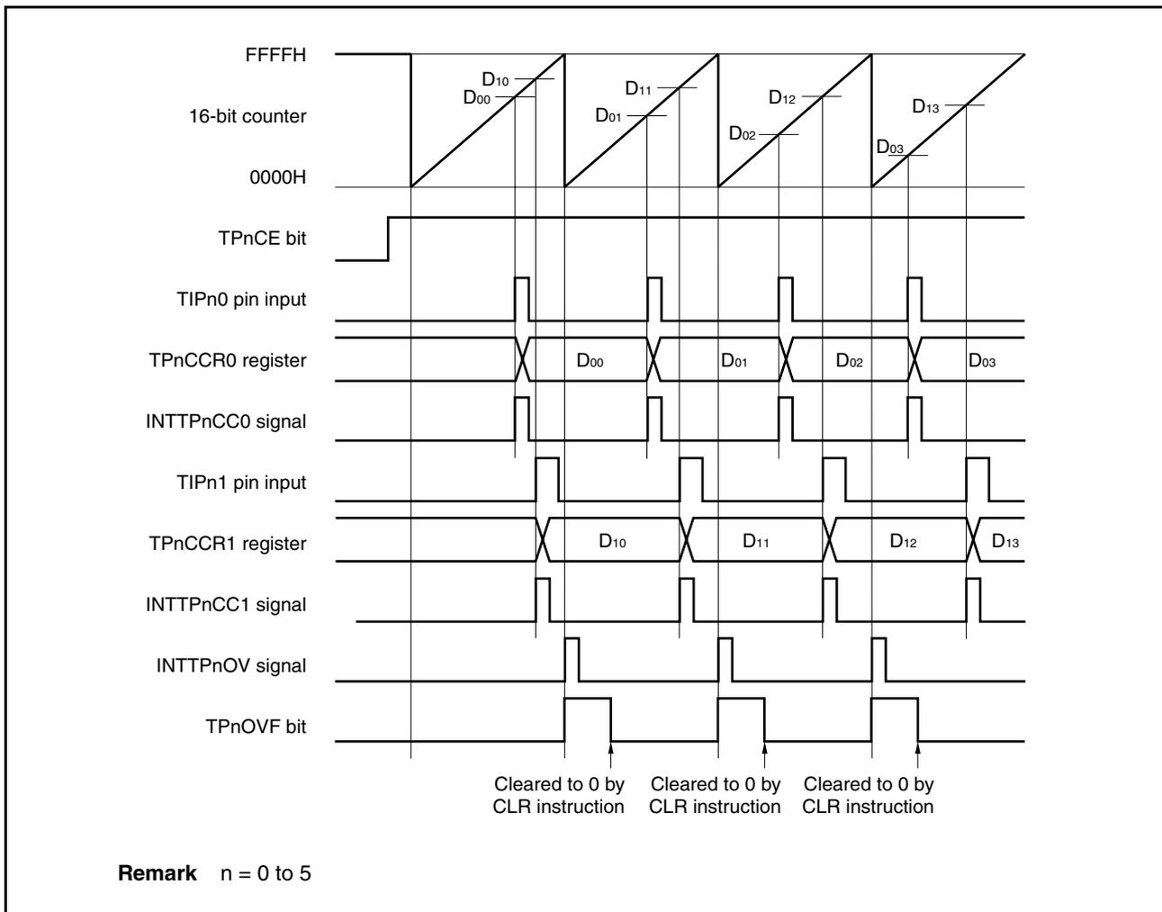
Figure 7-31. Register Setting in Free-Running Timer Mode (1/2)
