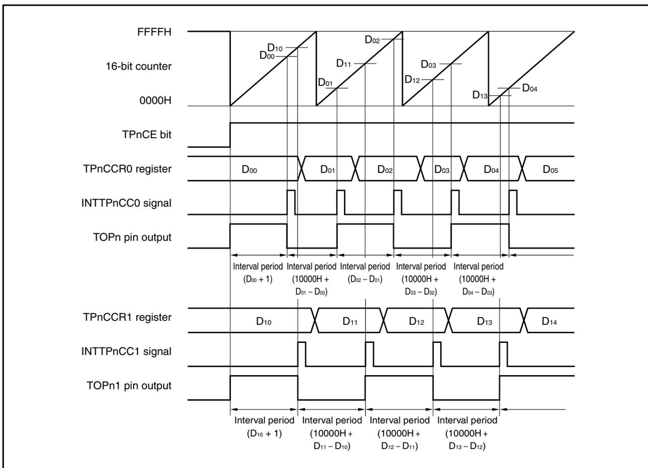
When performing an interval operation in the free-running timer mode, two intervals can be set with one channel.
