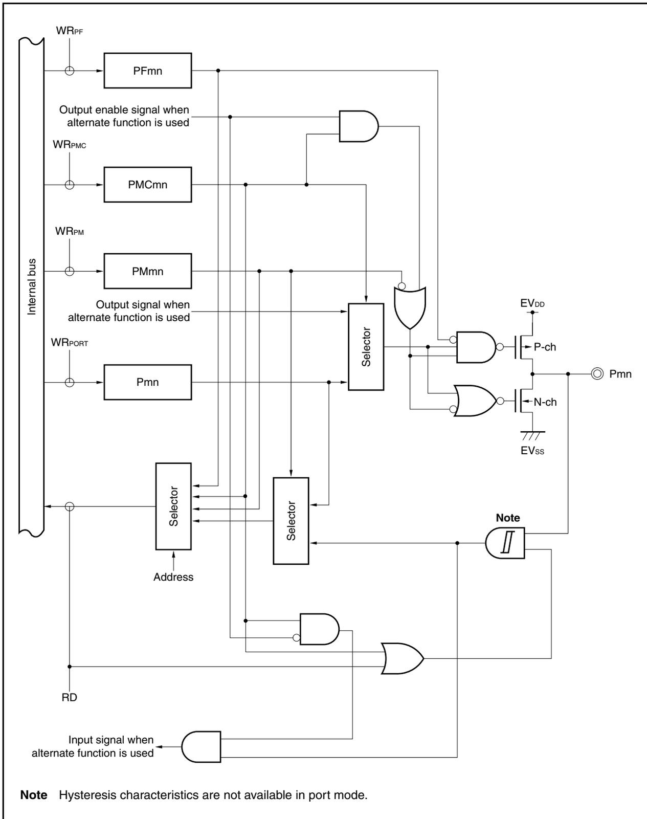
Figure 4-10. Block Diagram of Type G-1
