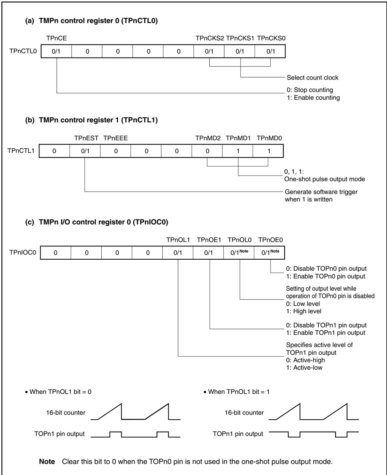
Figure 7-22. Register Setting for Operation in One-Shot Pulse Output Mode (2/2)
