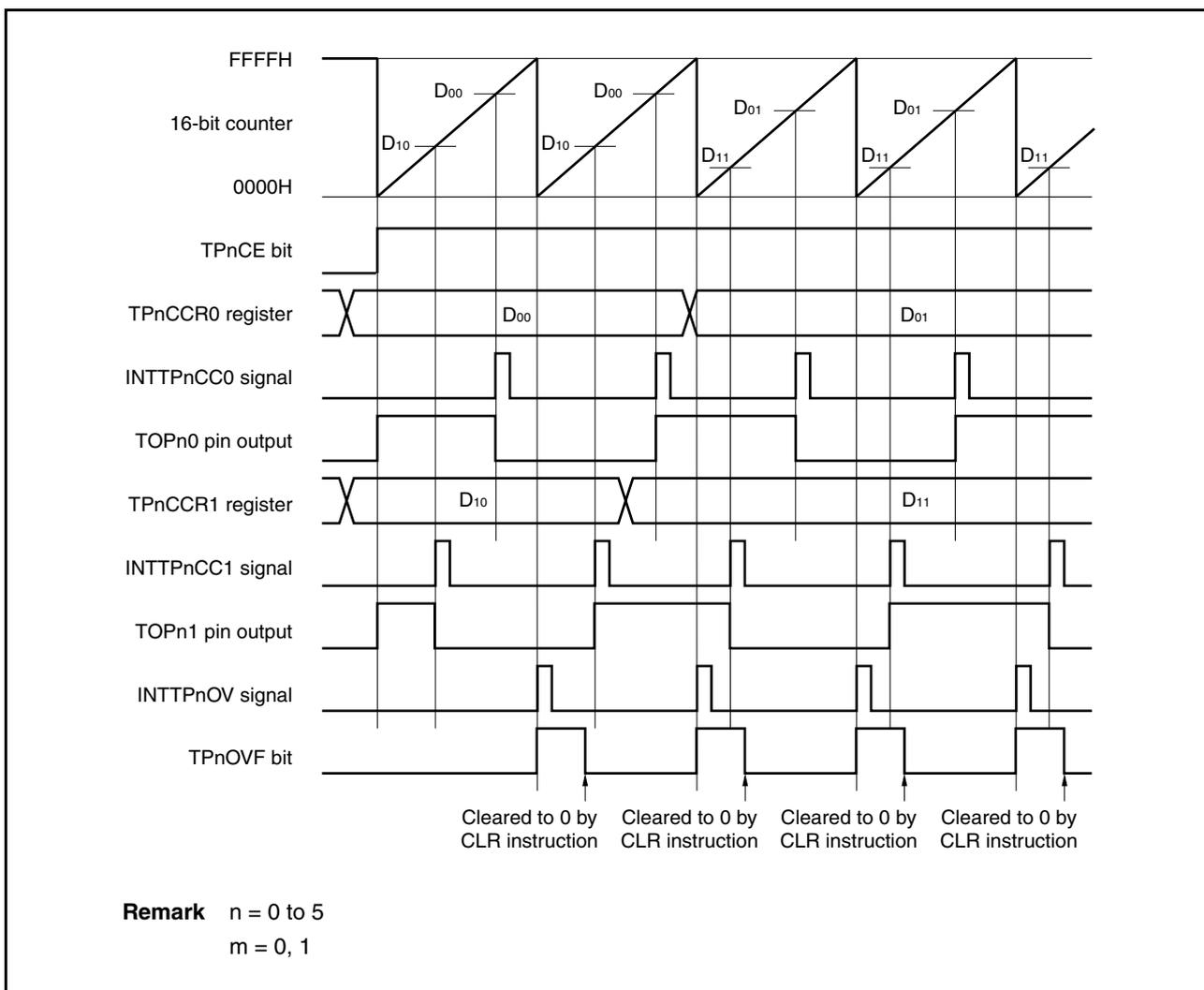
When the TPnCE bit is set to 1, the 16-bit counter starts counting. When the valid edge input to the TIPnm pin is detected, the count value of the 16-bit counter is stored in the TPnCCRm register, and a capture interrupt request signal (INTTPnCCm) is generated.
