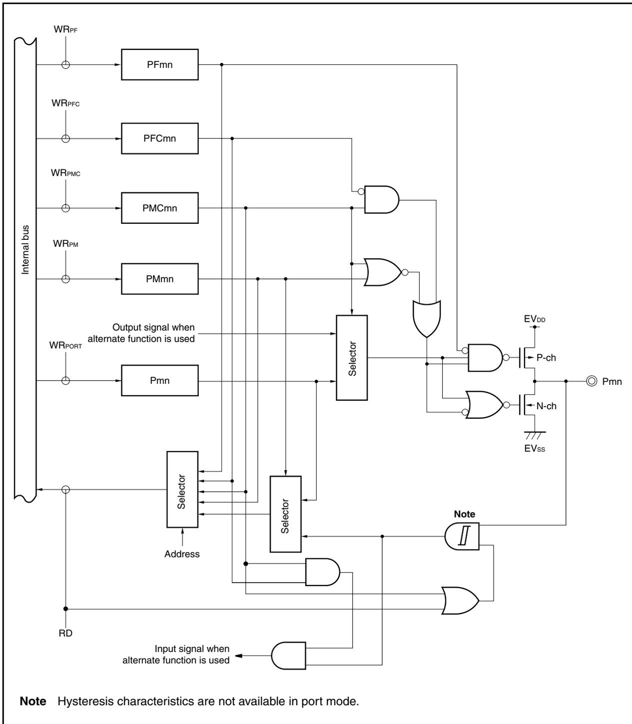
Figure 4-12. Block Diagram of Type G-3
