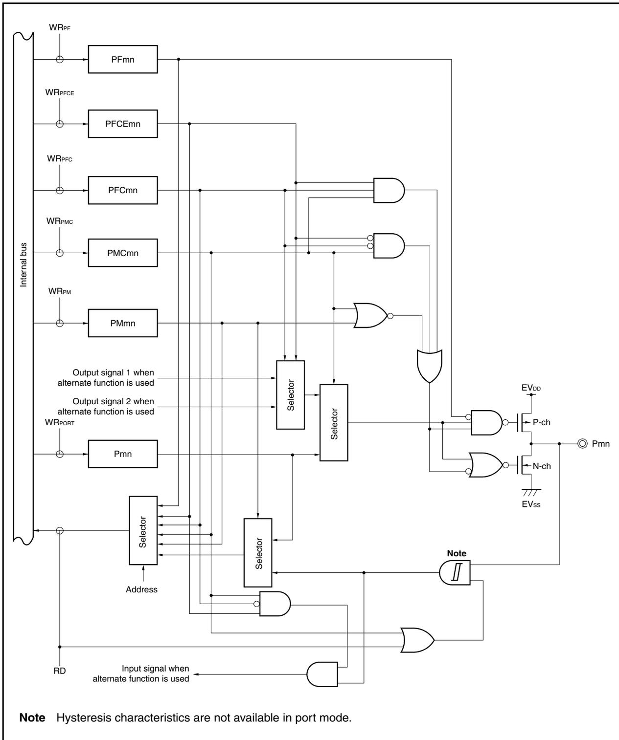
Figure 4-30. Block Diagram of Type U-14
