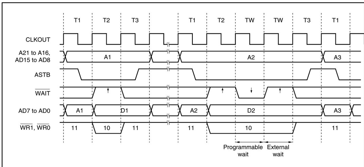
Figure 5-8. Multiplexed Bus Hold Timing (Bus Size: 16 Bits, 16-Bit Access)
