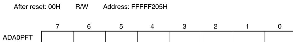
**Caution** When writing data to the ADA0PFT register in the following modes, stop the A/D conversion by clearing the AD0M0.ADA0CE bit to 0. After the data is written to the register, enable the A/D conversion again by setting the ADA0CE bit to 1.
