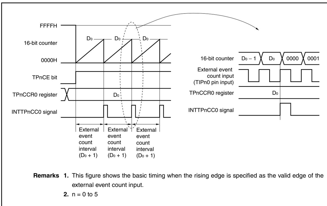
When the TPnCE bit is set to 1, the value of the 16-bit counter is cleared from FFFFH to 0000H. The counter counts each time the valid edge of external event count input is detected. Additionally, the set value of the TPnCCR0 register is transferred to the CCR0 buffer register.
