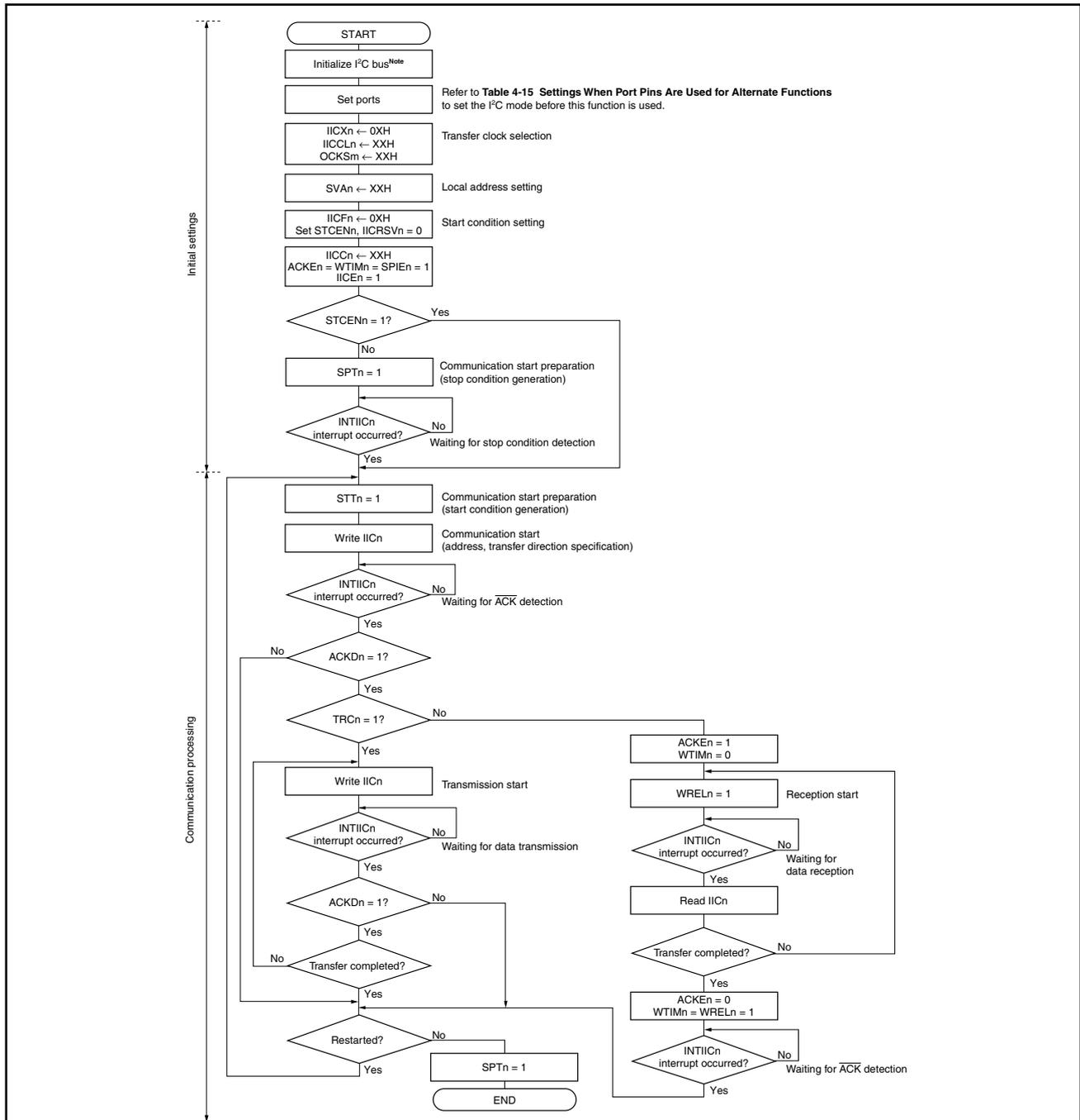
**Note** Release the I<sup>2</sup>C0n bus (SCL0n, SDA0n pins = high level) in conformity with the specifications of the product in communication.
