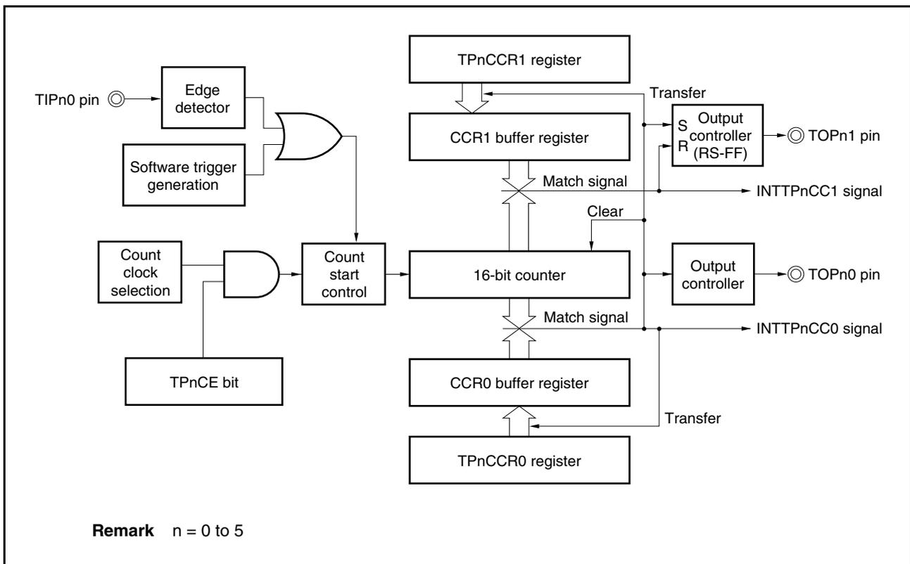
Figure 7-17. Basic Timing in External Trigger Pulse Output Mode
