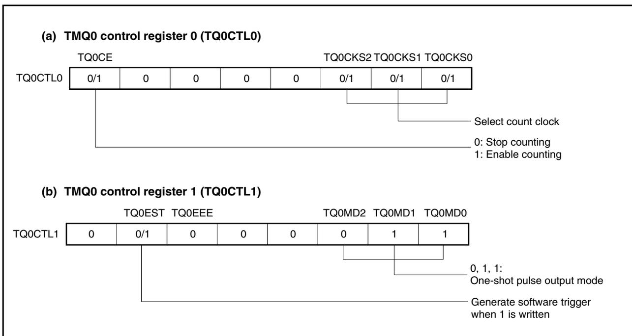
Figure 8-22. Register Setting for Operation in One-Shot Pulse Output Mode (2/3)
