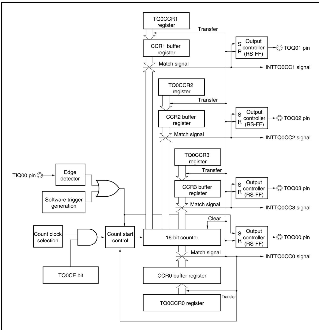
Figure 8-21. Basic Timing in One-Shot Pulse Output Mode
