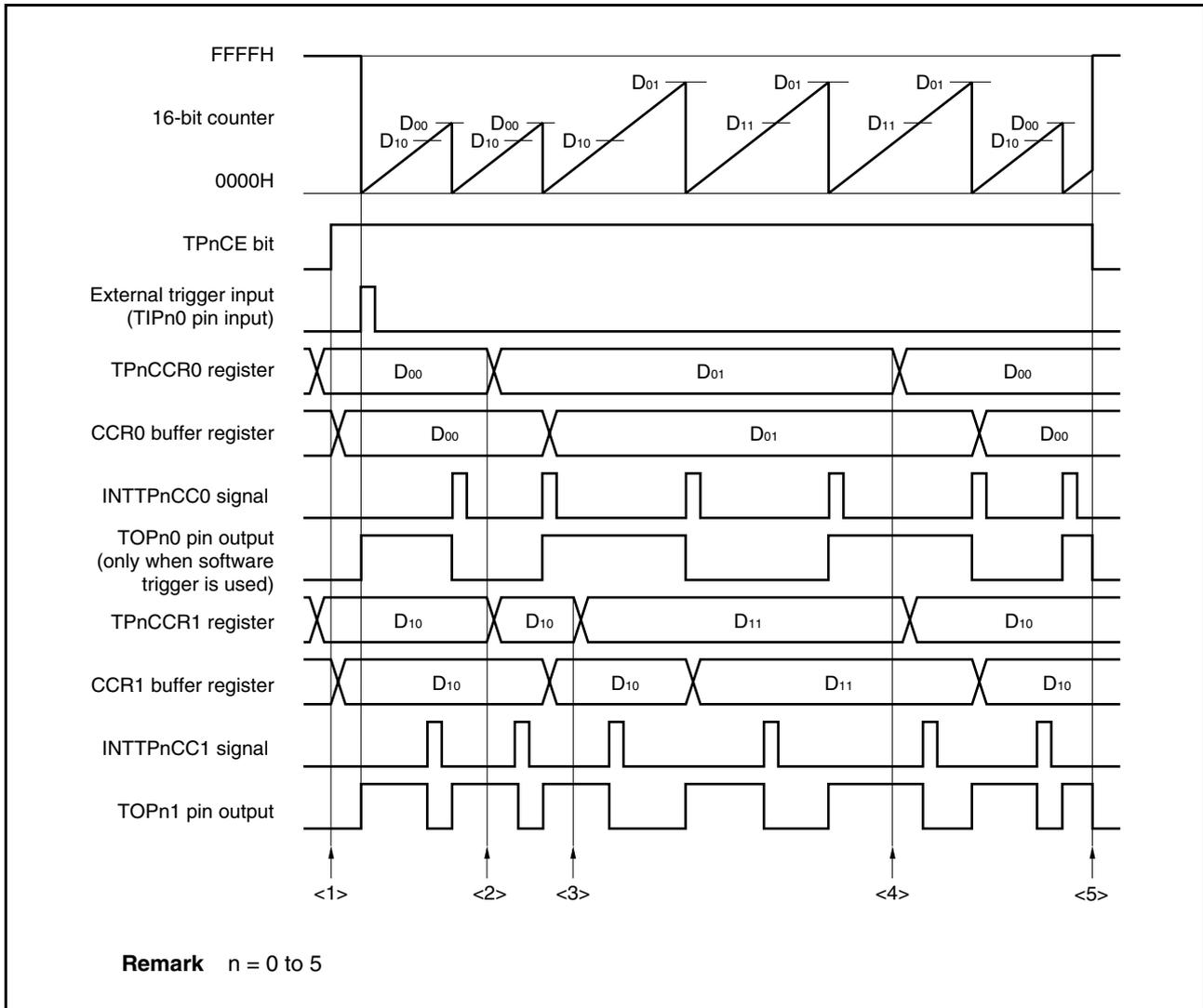
Figure 7-19. Software Processing Flow in External Trigger Pulse Output Mode (2/2)
