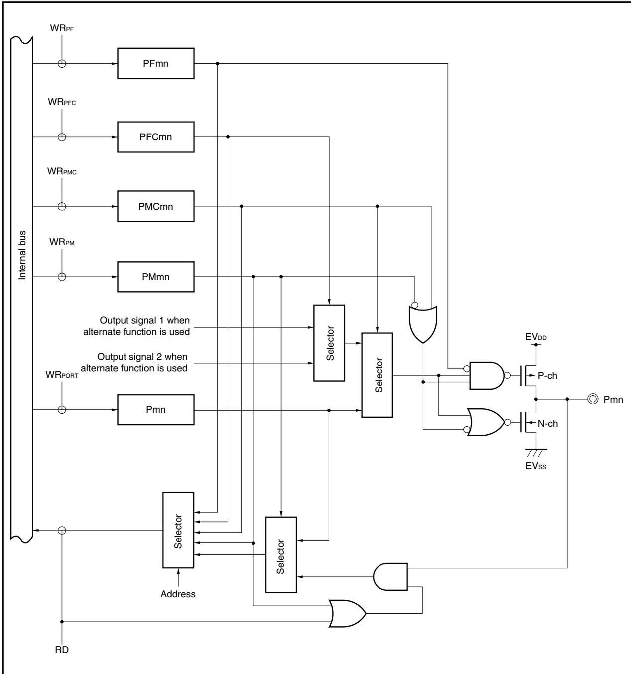
Figure 4-13. Block Diagram of Type G-5
