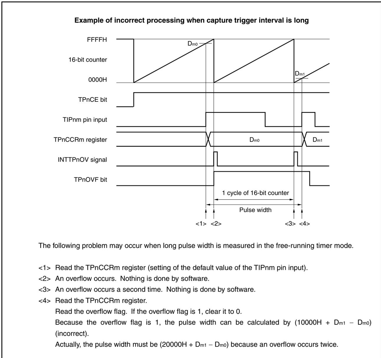
If an overflow occurs twice or more when the capture trigger interval is long, the correct pulse width may not be obtained.
