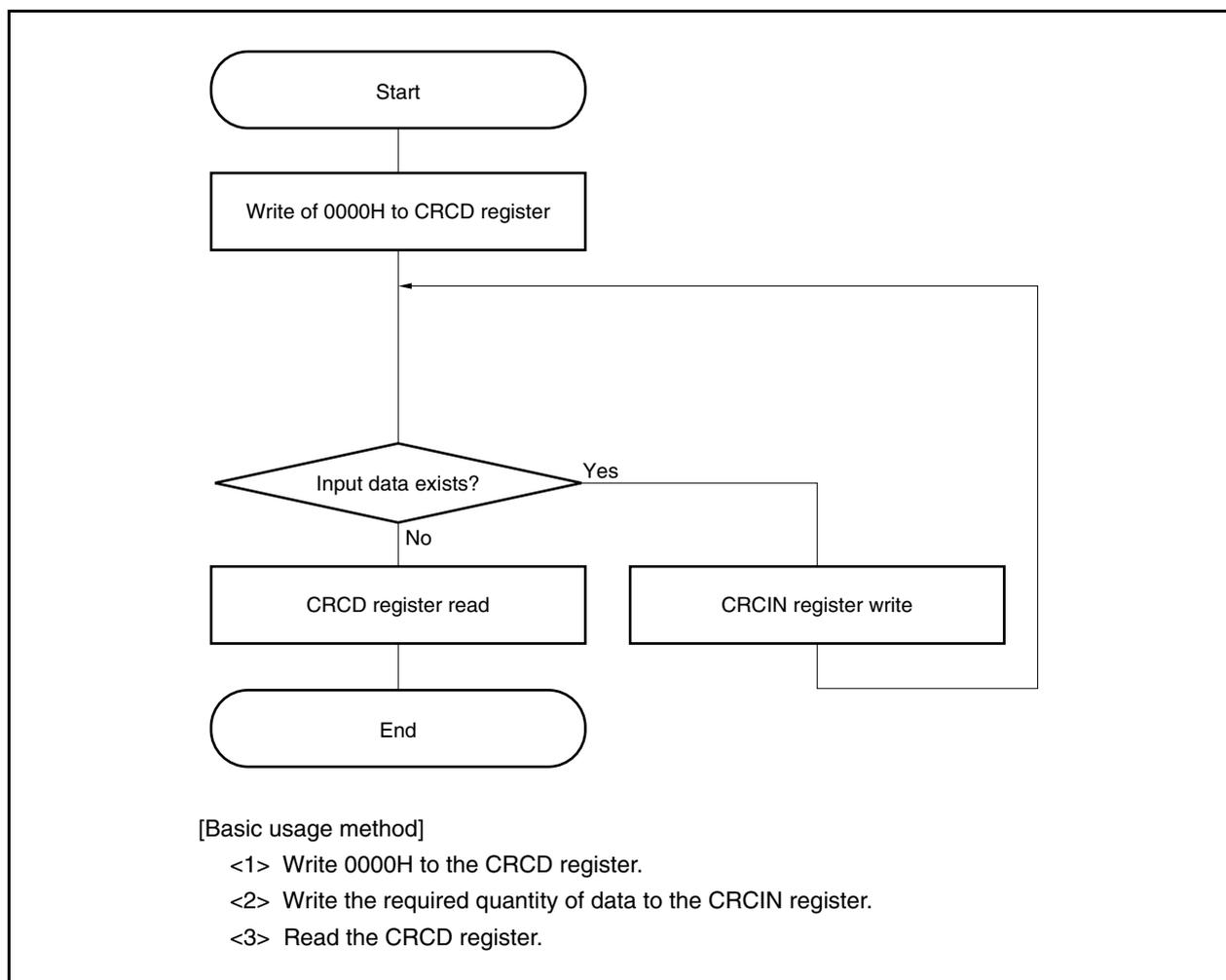
Communication errors can easily be detected if the CRC code is transmitted/received along with transmit/receive data when transmitting/receiving data consisting of several bytes.
