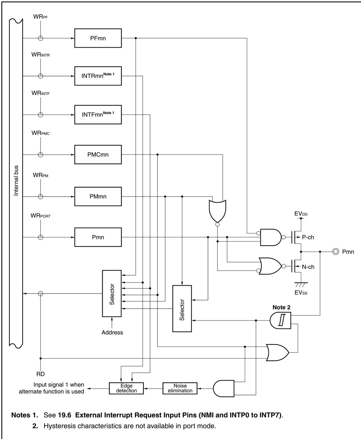
Figure 4-17. Block Diagram of Type N-1
