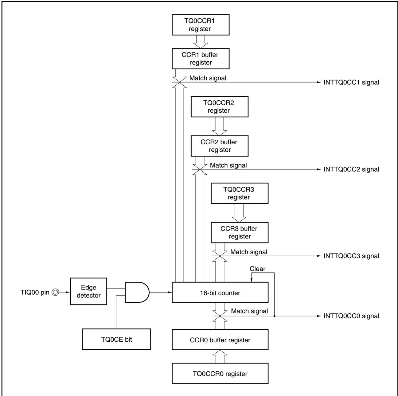
If the set value of the TQ0CCRk register is smaller than the set value of the TQ0CCR0 register, the INTTQ0CCk signal is generated once per cycle.
