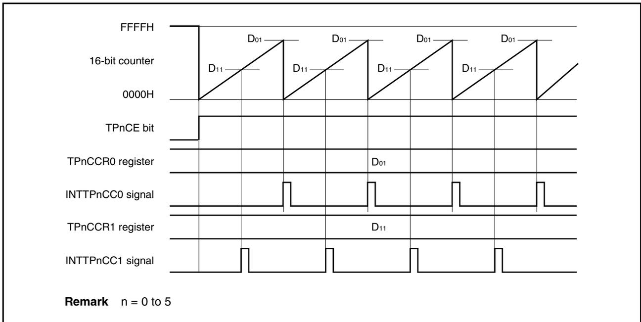
If the set value of the TPnCCR1 register is greater than the set value of the TPnCCR0 register, the INTTPnCC1 signal is not generated because the count value of the 16-bit counter and the value of the TPnCCR1 register do not match.
