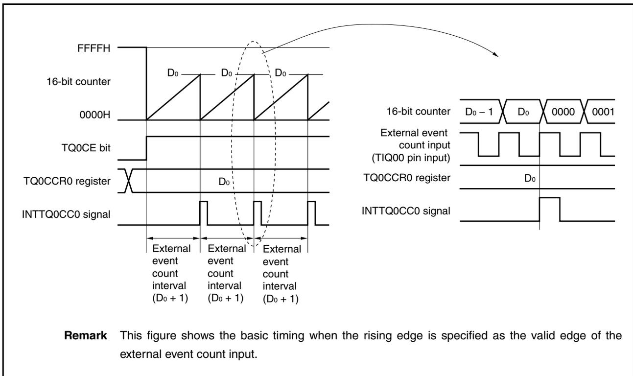
When the TQ0CE bit is set to 1, the value of the 16-bit counter is cleared from FFFFH to 0000H. The counter counts each time the valid edge of external event count input is detected. Additionally, the set value of the TQ0CCR0 register is transferred to the CCR0 buffer register.
