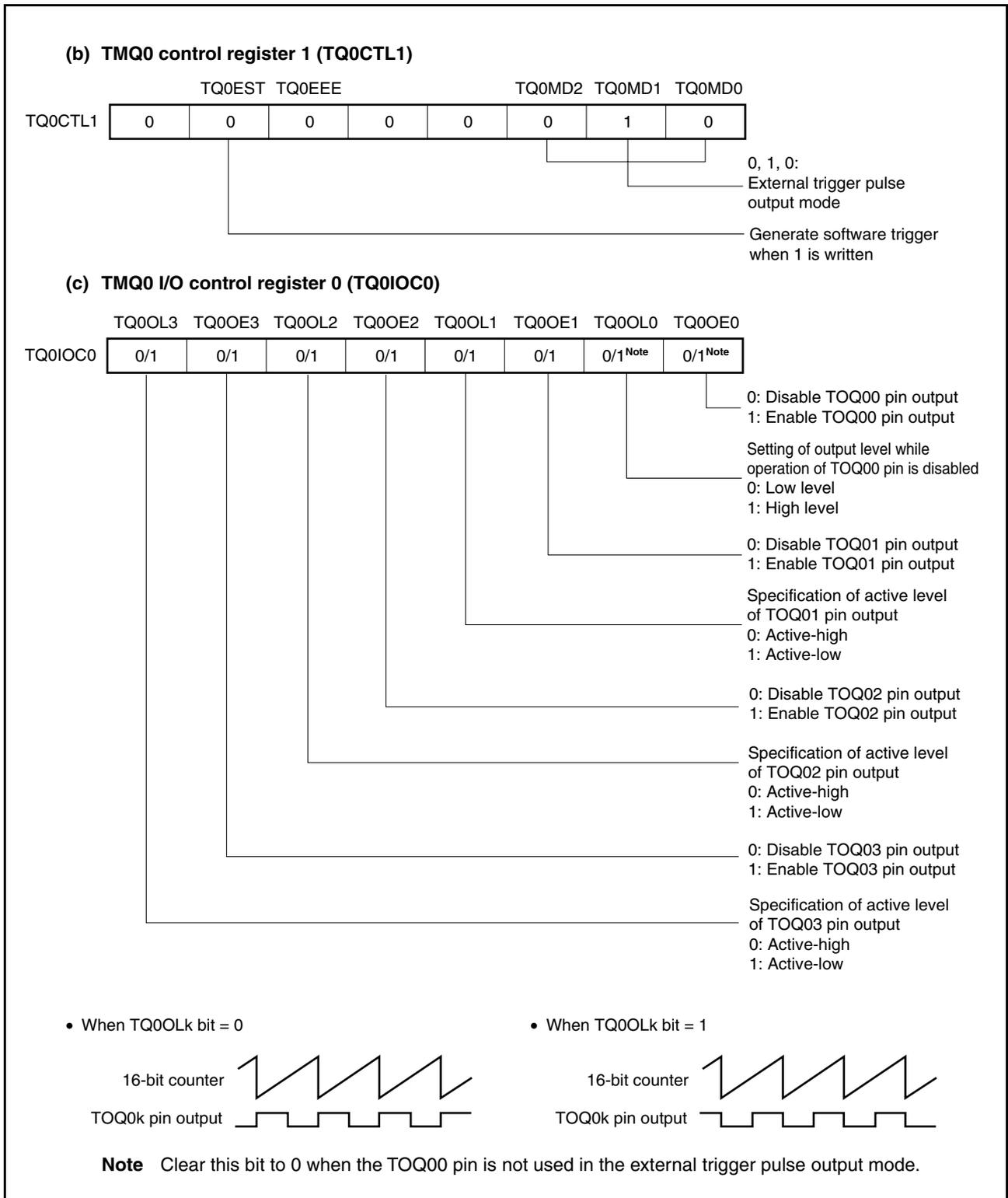
(1) Operation flow in external trigger pulse output mode
