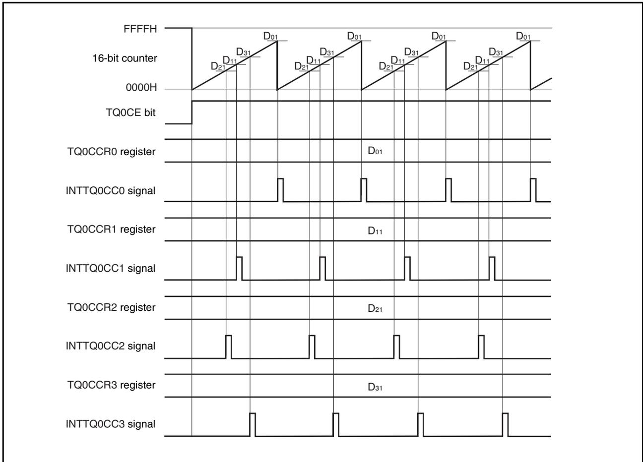
If the set value of the TQ0CCRk register is greater than the set value of the TQ0CCR0 register, the INTTQ0CCk signal is not generated because the count value of the 16-bit counter and the value of the TQ0CCRk register do not match.
