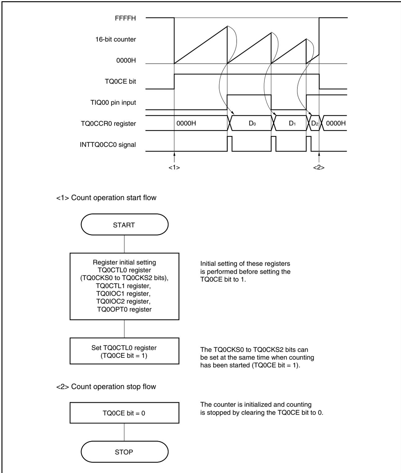
**(2) Operation timing in pulse width measurement mode****(a) Clearing overflow flag**
