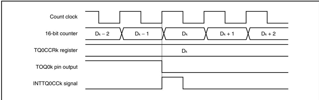
Usually, the INTTQ0CCK signal is generated when the 16-bit counter counts up next time after its count value matches the value of the TQ0CCRk register.
