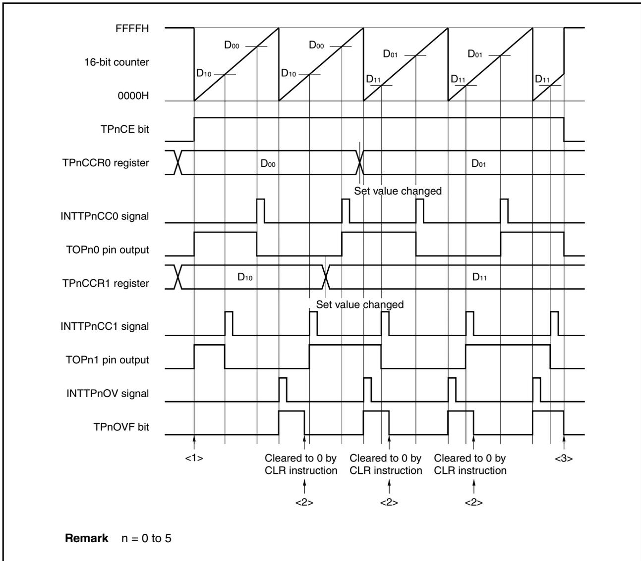
Figure 7-32. Software Processing Flow in Free-Running Timer Mode (Compare Function) (2/2)
