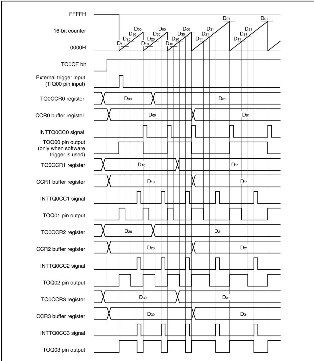
In order to transfer data from the TQ0CCR<sub>m</sub> register to the CCR<sub>m</sub> buffer register, the TQ0CCR1 register must be written.
