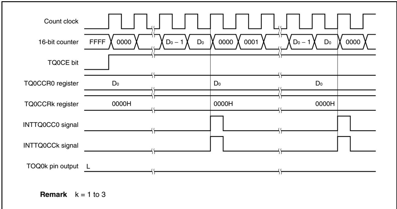
To output a 100% waveform, set a value of (set value of TQ0CCR0 register + 1) to the TQ0CCRk register. If the set value of the TQ0CCR0 register is FFFFH, 100% output cannot be produced.
