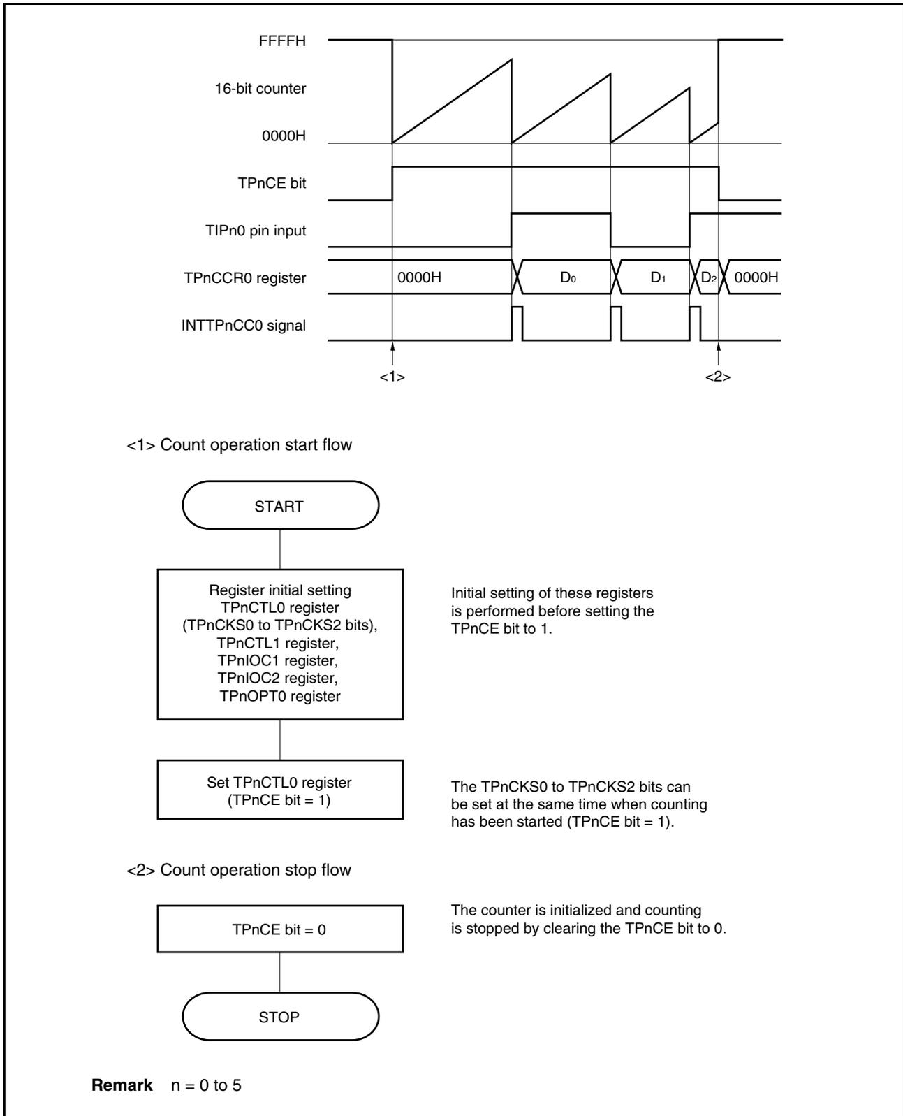
(2) Operation timing in pulse width measurement mode
