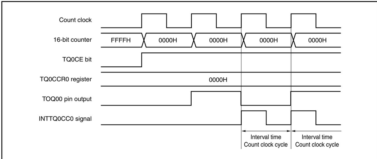
**(b) Operation if TQ0CCR0 register is set to FFFFH**
