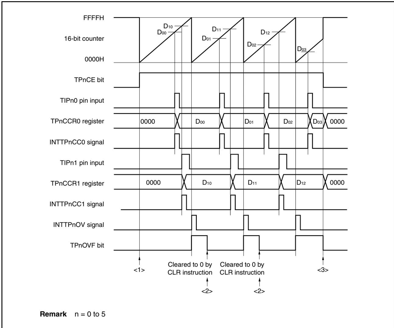
Figure 7-33. Software Processing Flow in Free-Running Timer Mode (Capture Function) (2/2)
