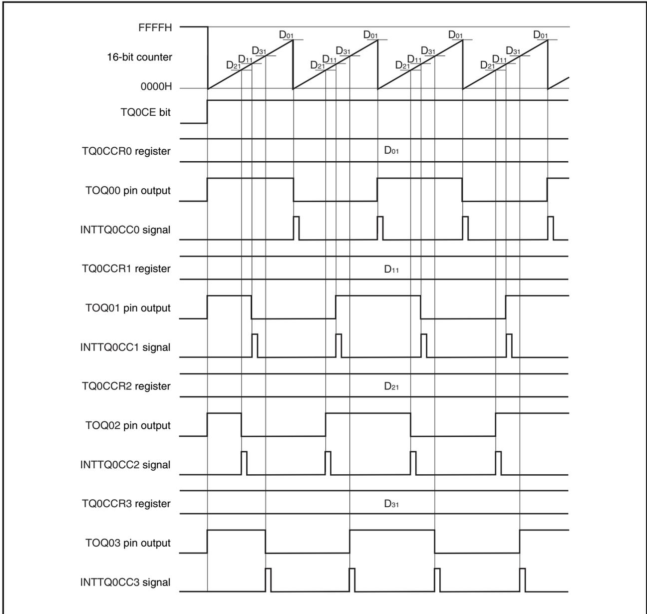
If the set value of the TQ0CCRk register is greater than the set value of the TQ0CCR0 register, the count value of the 16-bit counter does not match the value of the TQ0CCRk register. Consequently, the INTTQ0CCk signal is not generated, nor is the output of the TOQ0k pin changed.
