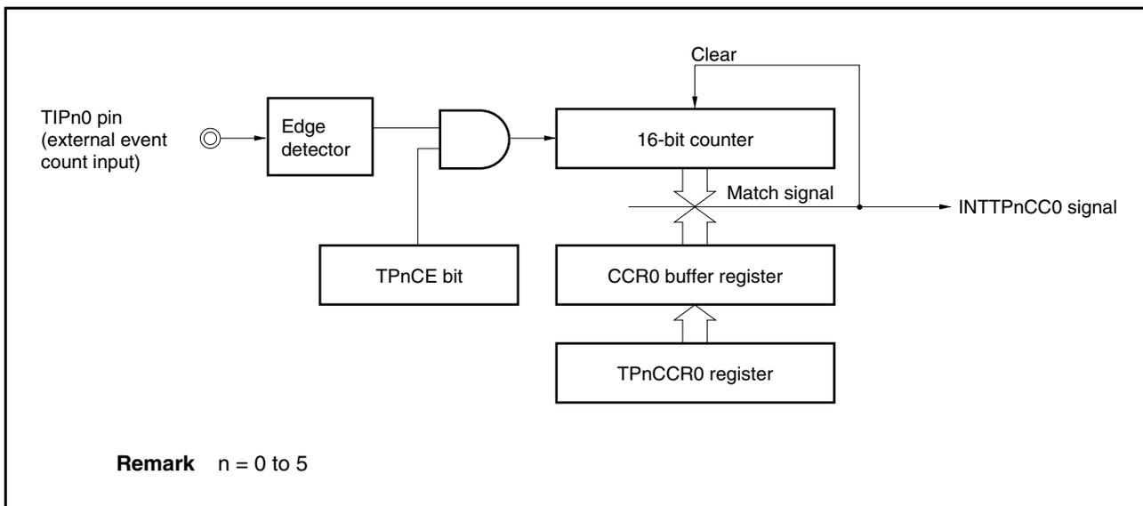
**Figure 7-10. Basic Timing in External Event Count Mode**
