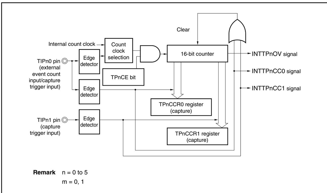
Figure 7-35. Basic Timing in Pulse Width Measurement Mode
