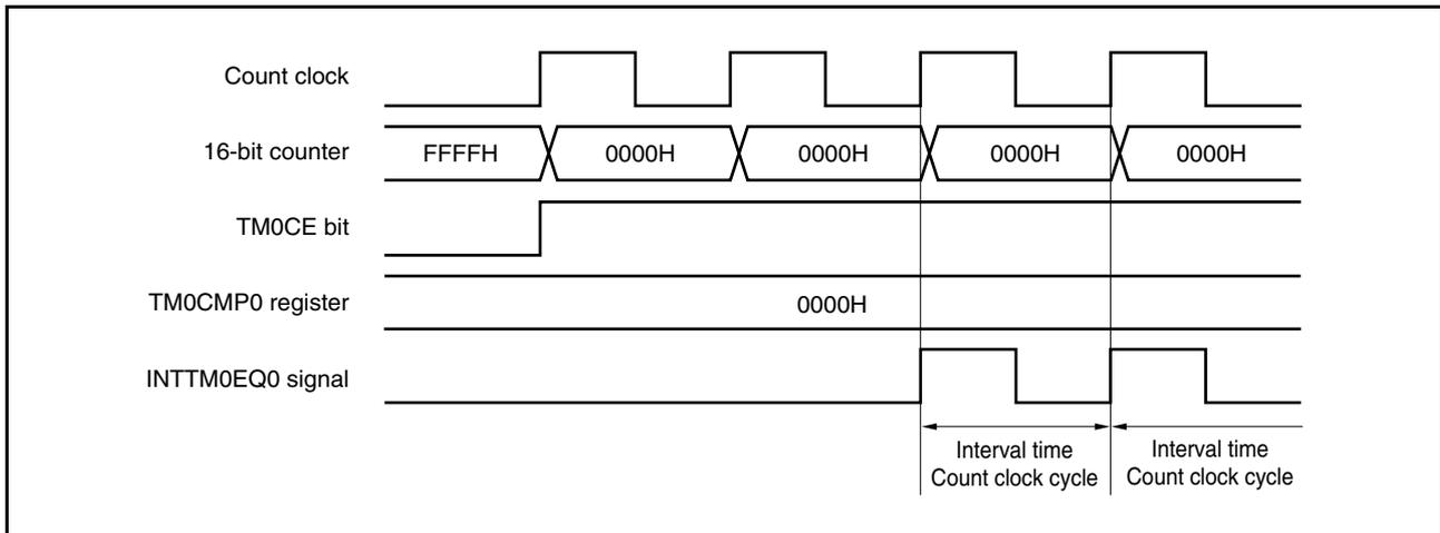
**(b) Operation if TM0CMP0 register is set to N**
