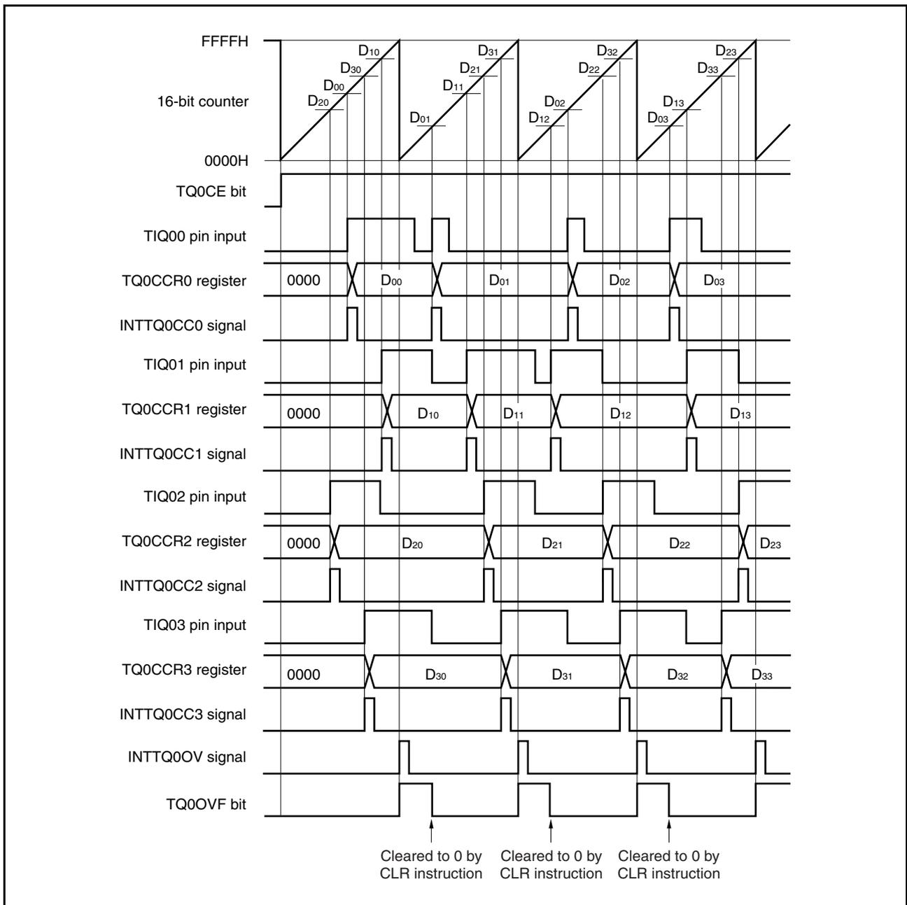
Figure 8-31. Register Setting in Free-Running Timer Mode (1/3)
