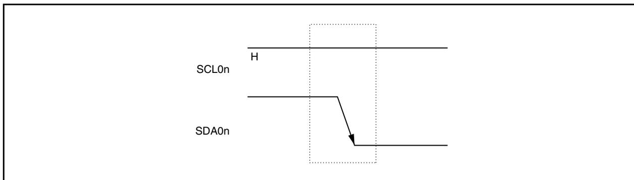
A start condition is output when the IICn.STTn bit is set (1) after a stop condition has been detected (IICn.SPDn bit = 1). When a start condition is detected, the IICn.STDn bit is set (1) (n = 0 to 2).
