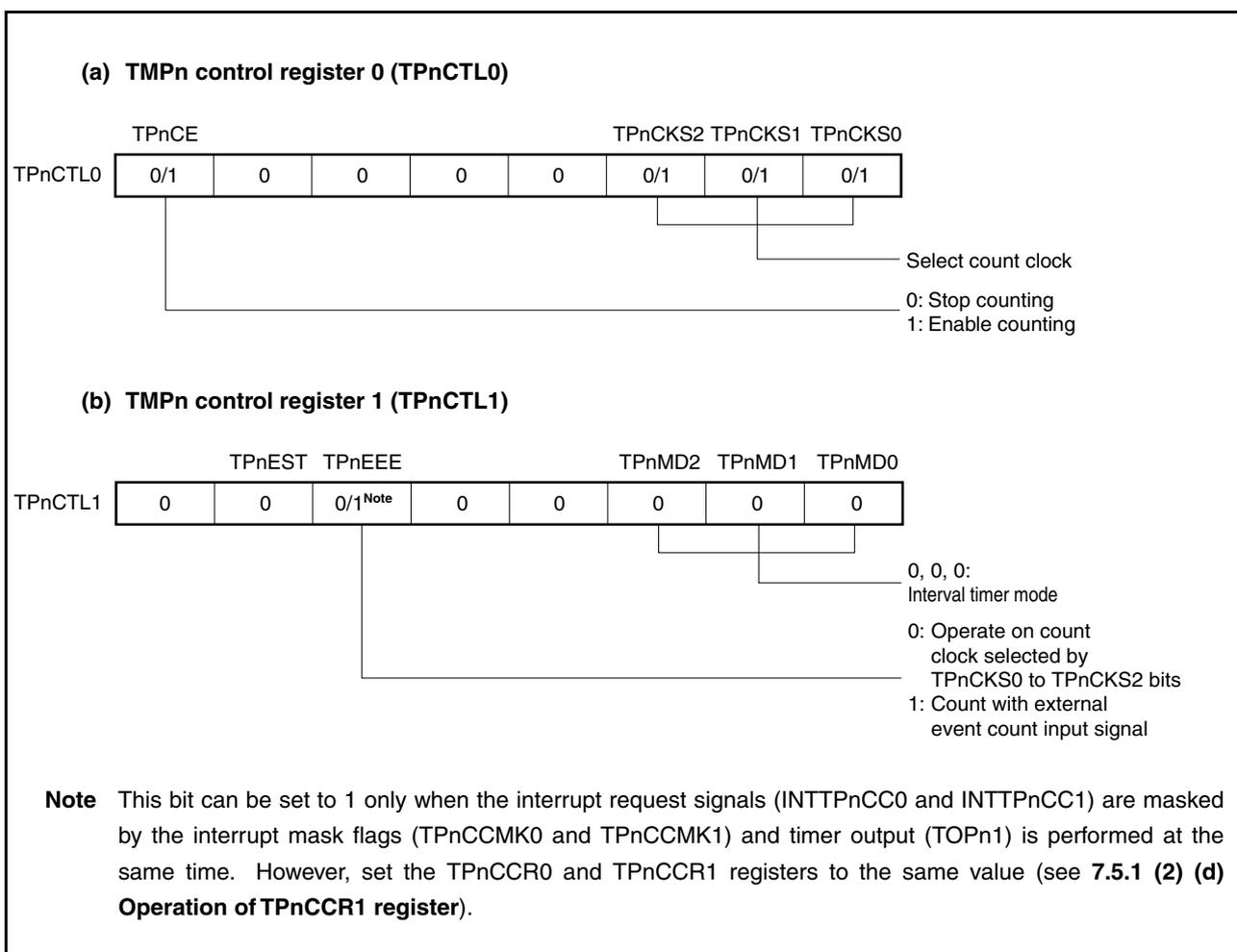
Figure 7-4. Register Setting for Interval Timer Mode Operation (2/2)
