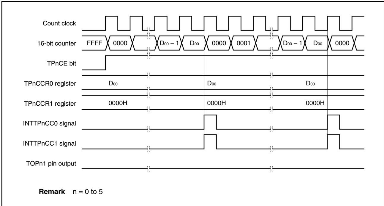
To output a 100% waveform, set a value of (set value of TPnCCR0 register + 1) to the TPnCCR1 register. If the set value of the TPnCCR0 register is FFFFH, 100% output cannot be produced.
