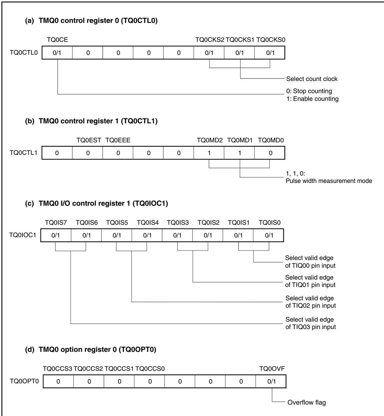
Figure 8-36. Register Setting in Pulse Width Measurement Mode (2/2)
