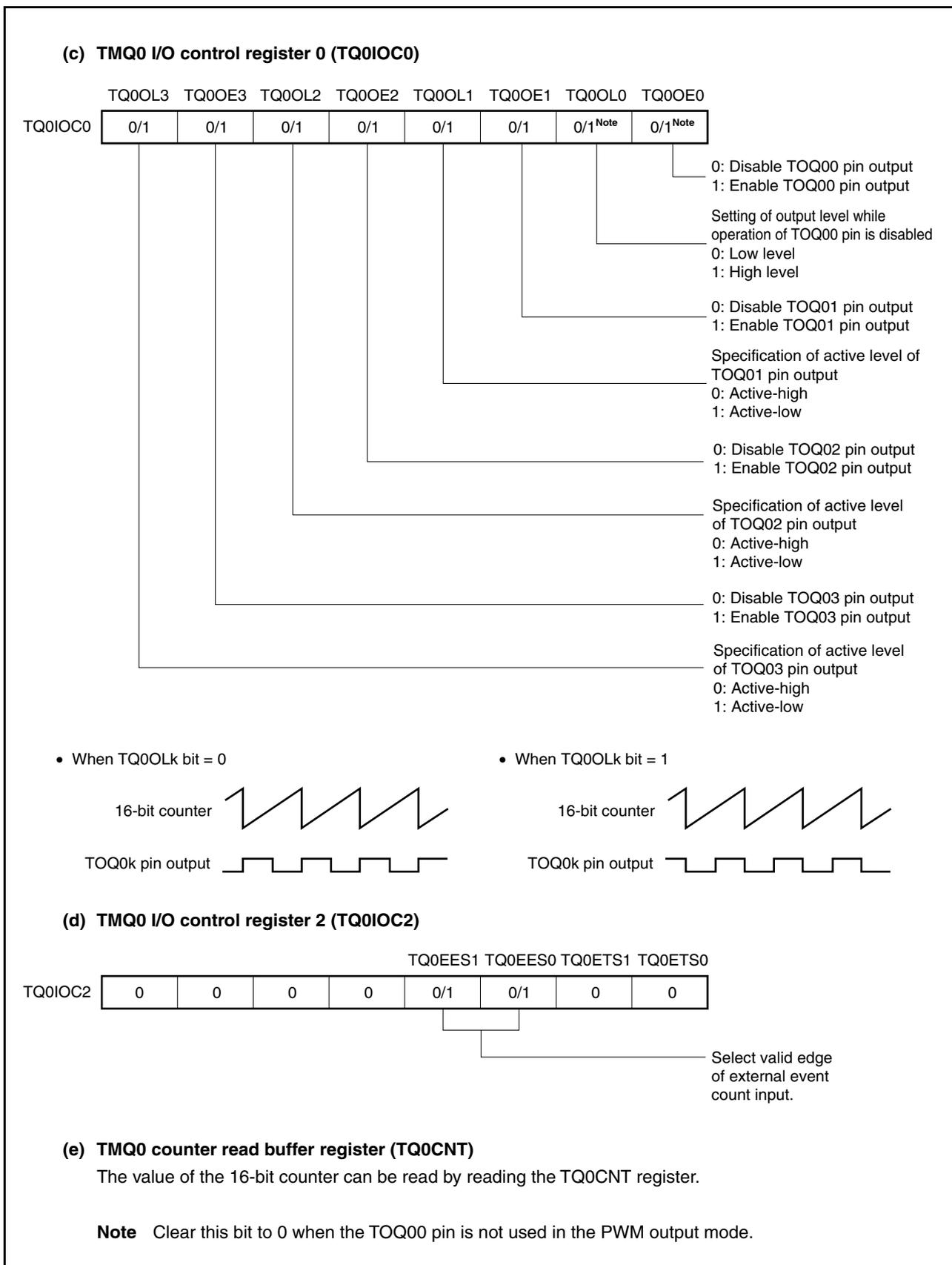
Figure 8-26. Register Setting for Operation in PWM Output Mode (3/3)
