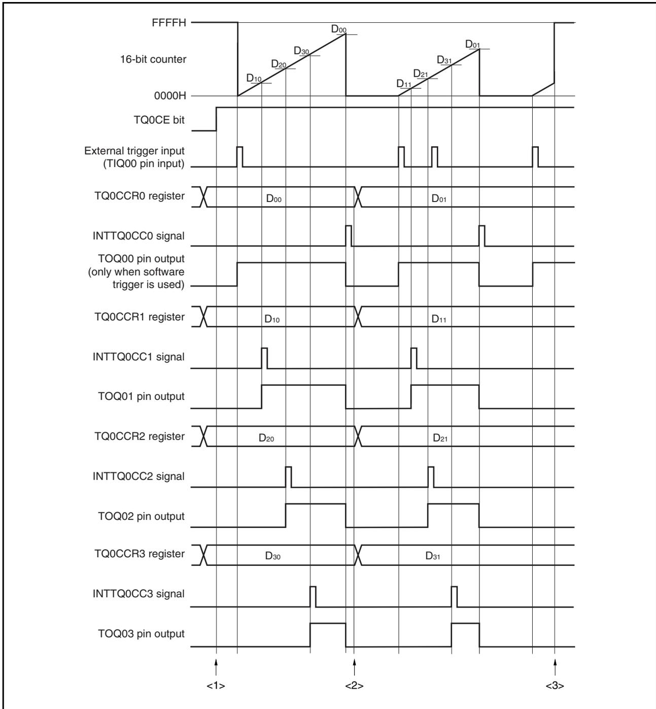
Figure 8-23. Software Processing Flow in One-Shot Pulse Output Mode (2/2)
