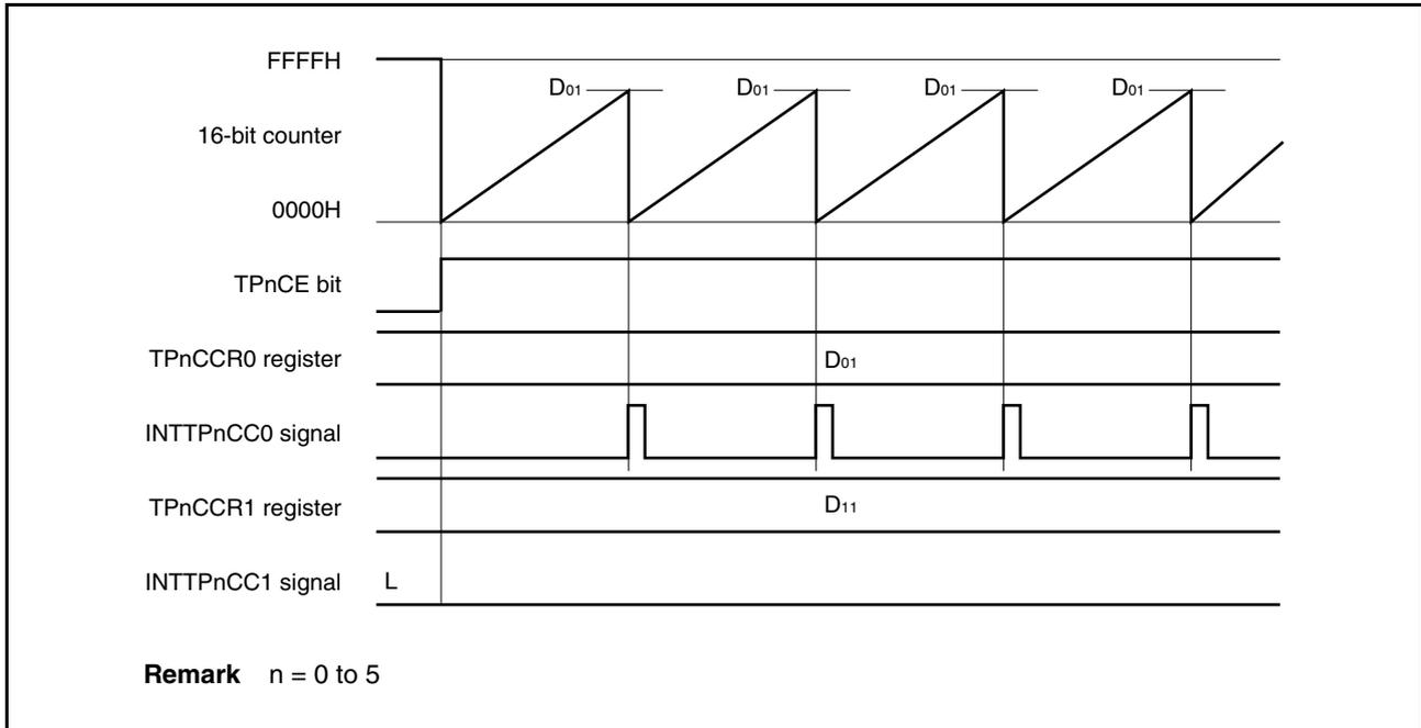
**7.5.3 External trigger pulse output mode (TPnMD2 to TPnMD0 bits = 010)**
