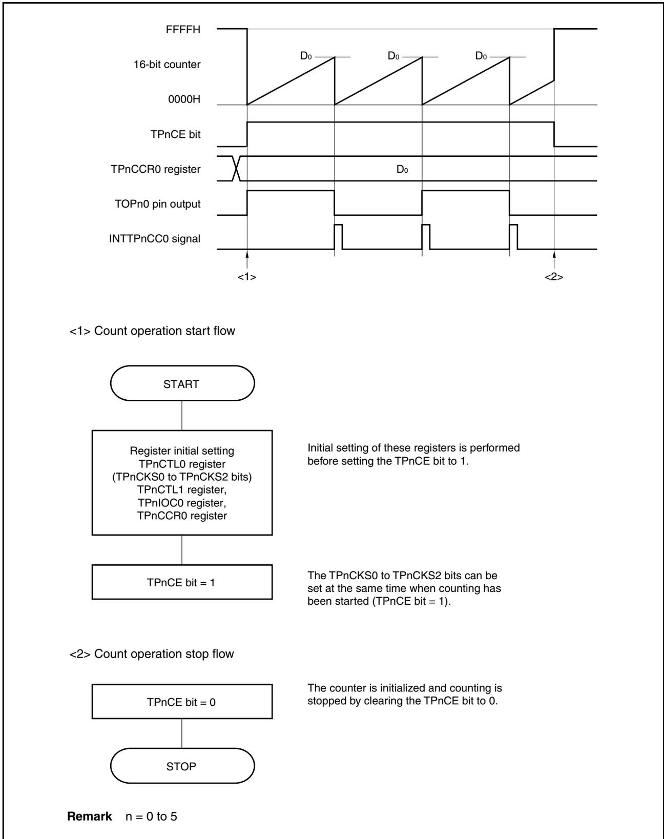
**(2) Interval timer mode operation timing****(a) Operation if TPnCCR0 register is set to 0000H**
