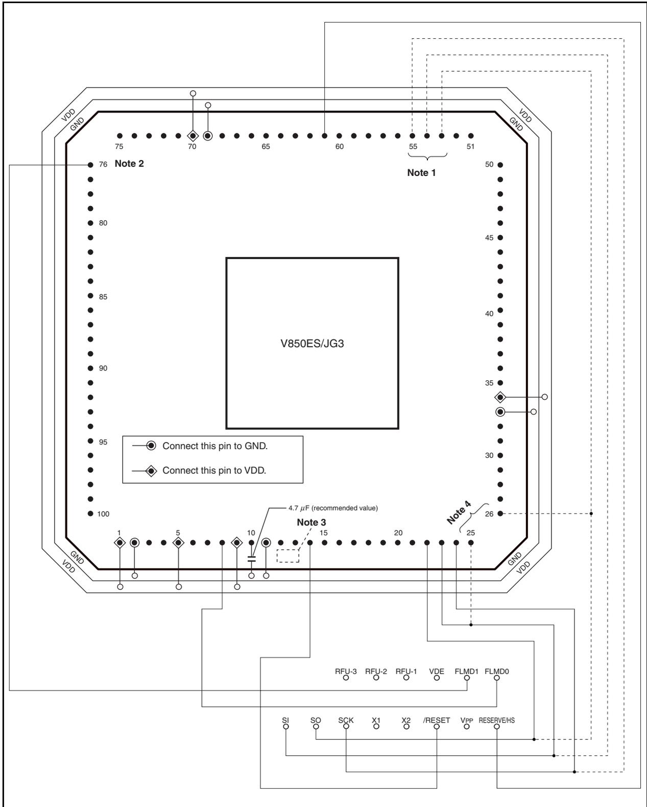
**Figure 27-6. Example of Wiring of V850ES/JG3 Flash Writing Adapter (FA-100GC-8EU-A)
