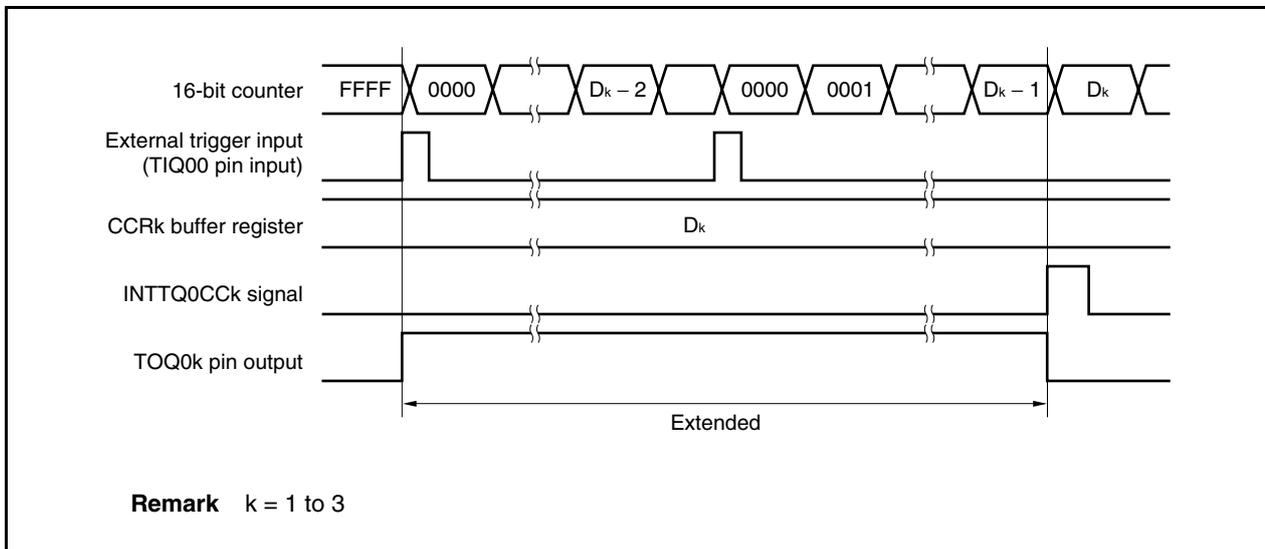
**(d) Conflict between trigger detection and match with CCR0 buffer register**
