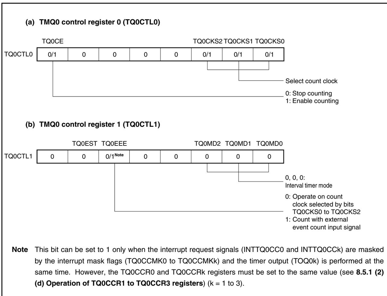
Figure 8-4. Register Setting for Interval Timer Mode Operation (2/2)
