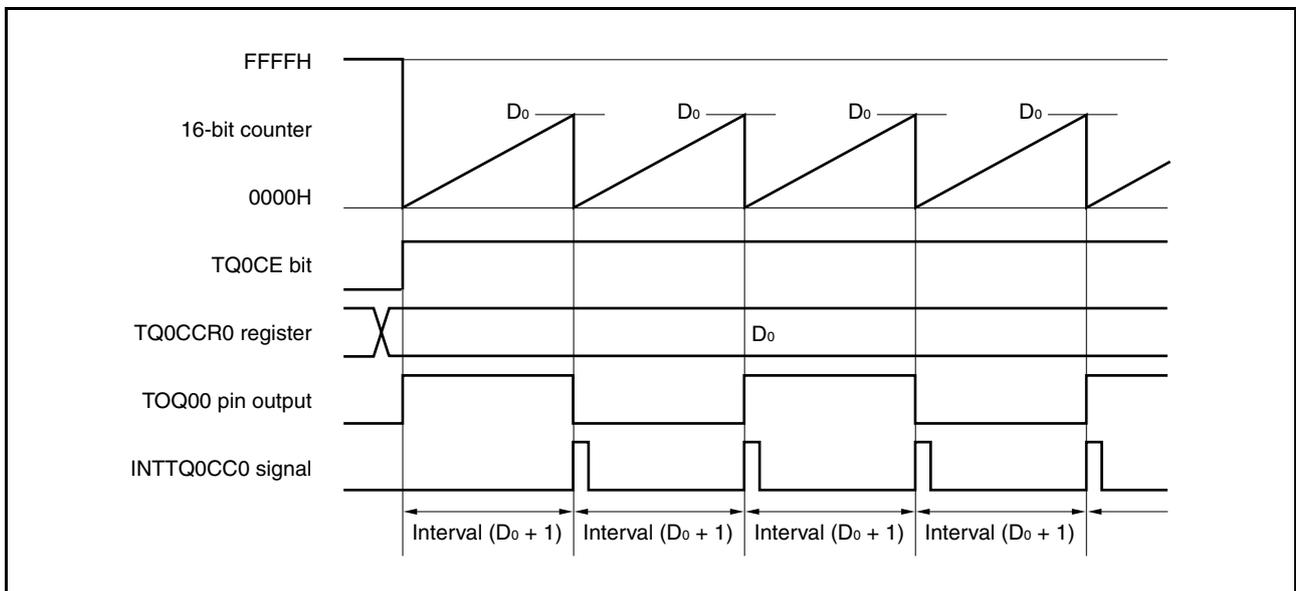
When the TQ0CE bit is set to 1, the value of the 16-bit counter is cleared from FFFFH to 0000H in synchronization with the count clock, and the counter starts counting. At this time, the output of the TOQ00 pin is inverted. Additionally, the set value of the TQ0CCR0 register is transferred to the CCR0 buffer register.
