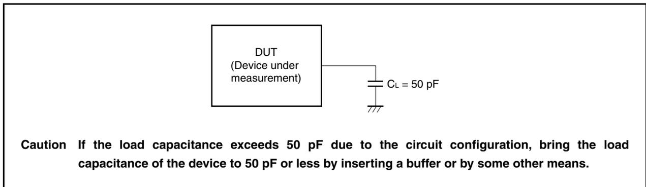
**CLKOUT Output Timing****( $T_A = -40$  to  $+85^\circ\text{C}$ ,  $V_{DD} = EV_{DD} = AV_{REF0} = AV_{REF1}$ ,  $V_{SS} = EV_{SS} = AV_{SS} = 0\text{ V}$ )**
