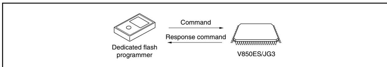
The following shows the commands for flash memory control in the V850ES/JG3. All of these commands are issued from the dedicated flash programmer, and the V850ES/JG3 performs the processing corresponding to the commands.
