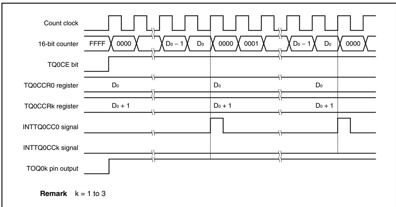
**(c) Generation timing of compare match interrupt request signal (INTTQ0CCK)**
