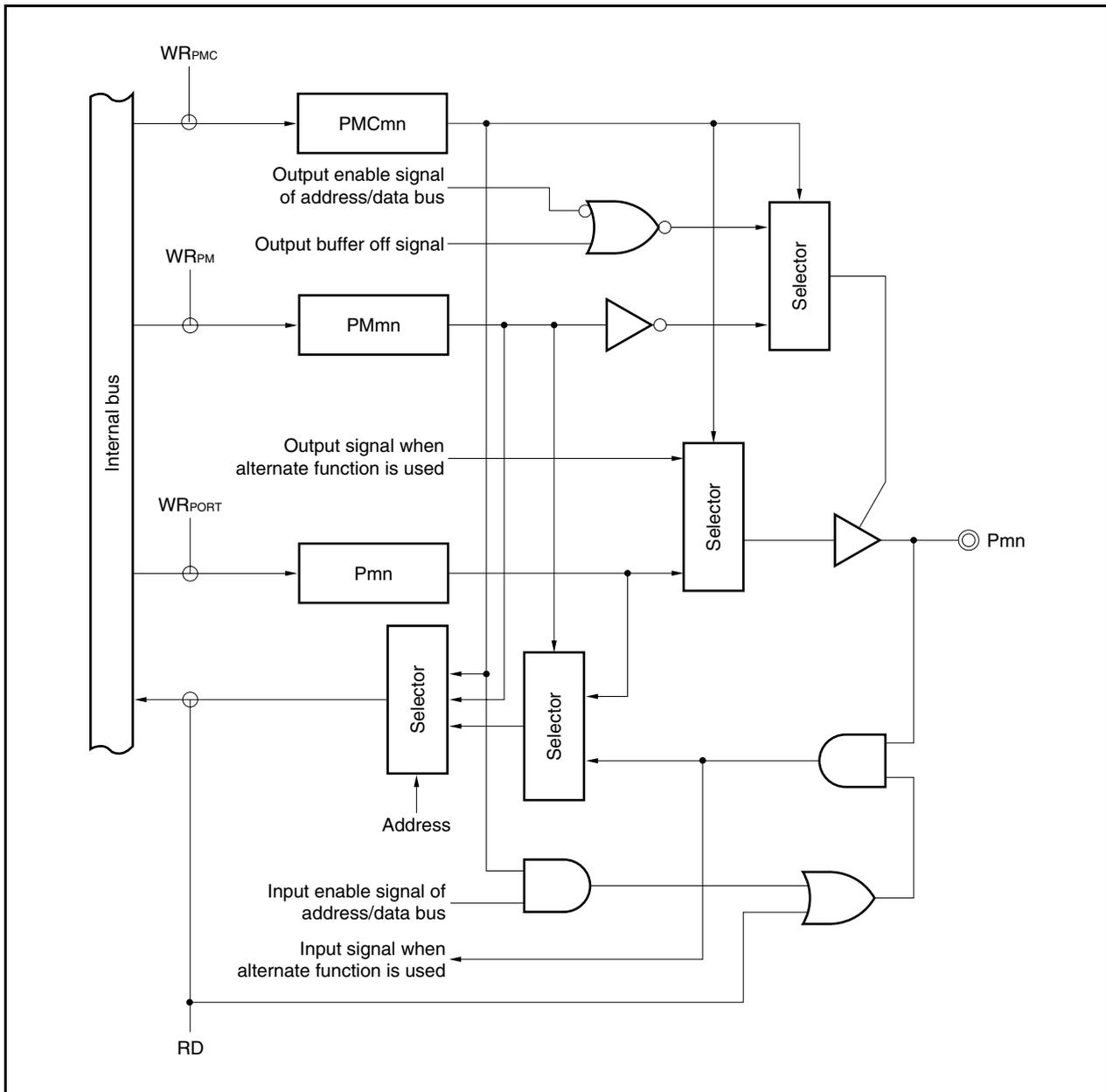
Figure 4-9. Block Diagram of Type E-3
