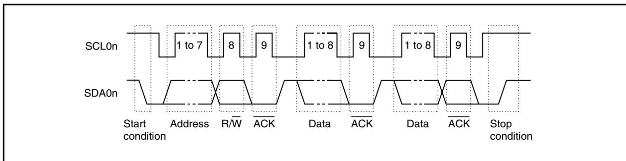
The master device generates the start condition, slave address, and stop condition.
