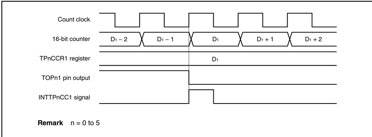
Usually, the INTTPnCC1 signal is generated in synchronization with the next counting up after the count value of the 16-bit counter matches the value of the TPnCCR1 register.
