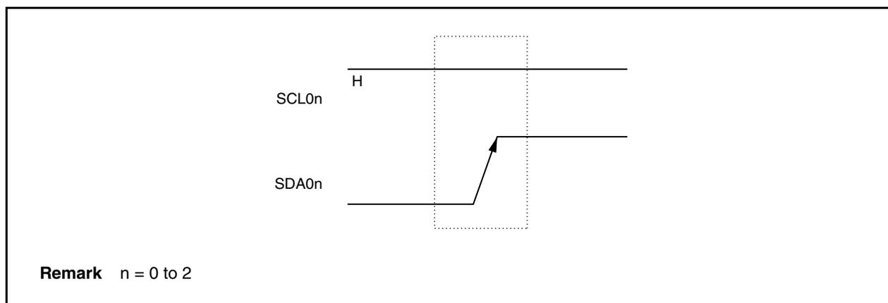
A stop condition is generated when the IICCn.SPTn bit is set to 1. When the stop condition is detected, the IICSn.SPDn bit is set to 1 and the interrupt request signal (INTIICn) is generated when the IICCn.SPIEn bit is set to 1 (n = 0 to 2).
