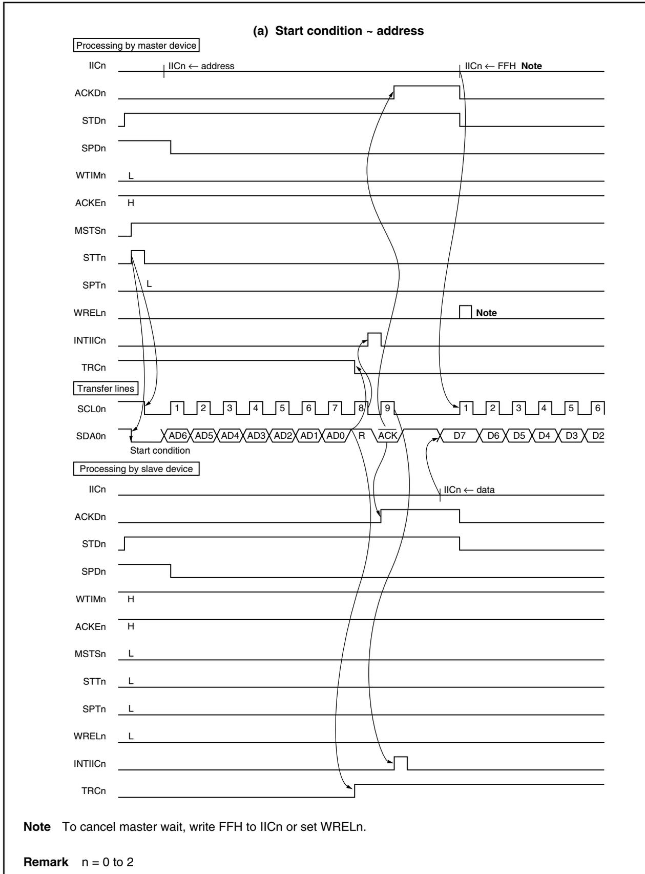
**Figure 17-24. Example of Slave to Master Communication**
