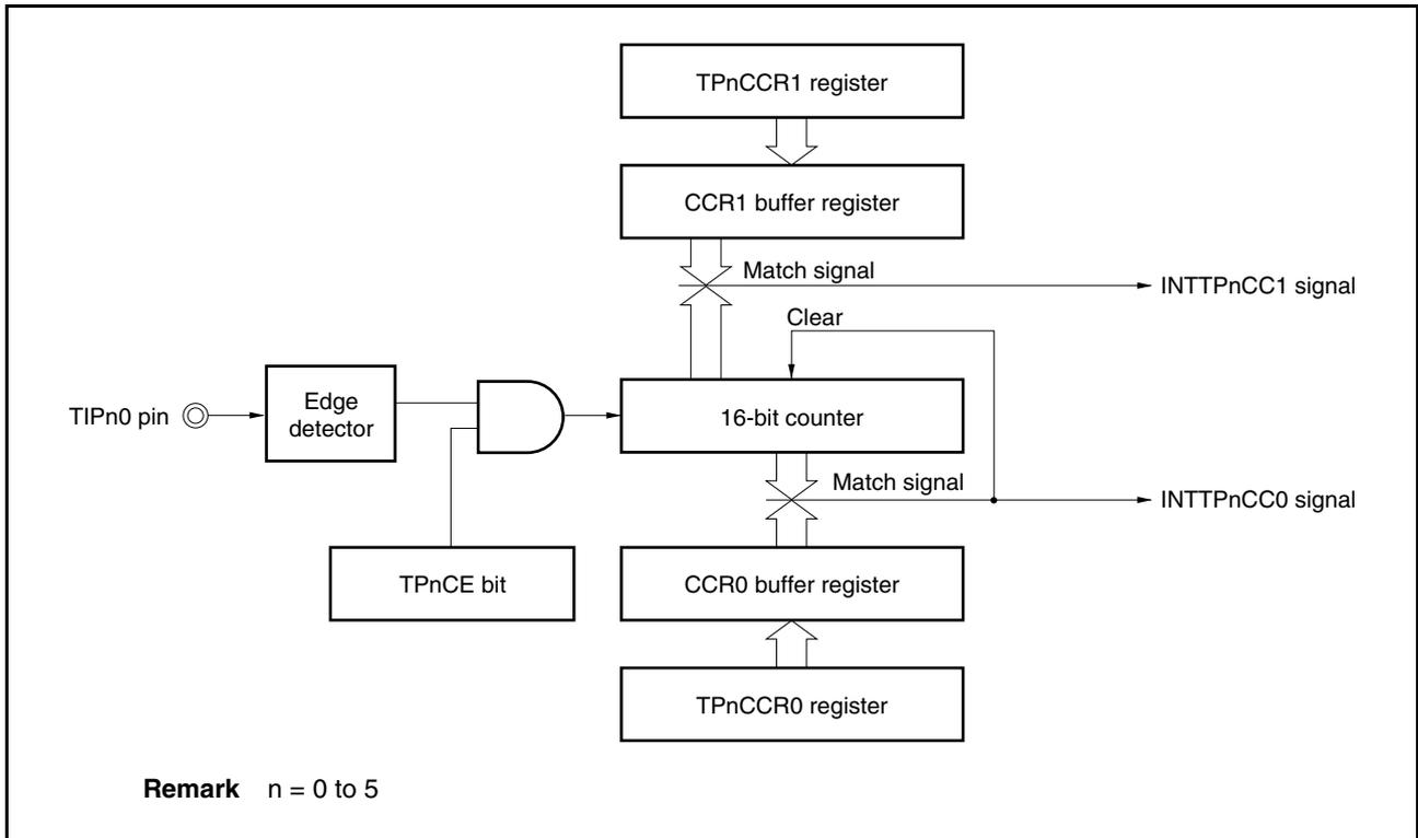
If the set value of the TPnCCR1 register is smaller than the set value of the TPnCCR0 register, the INTTPnCC1 signal is generated once per cycle.
