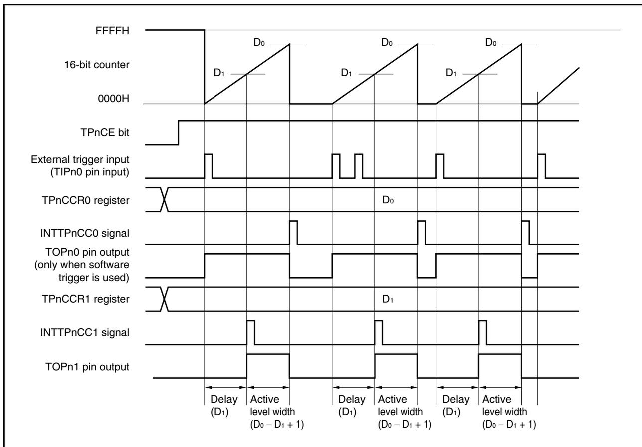
When the TPnCE bit is set to 1, 16-bit timer/event counter P waits for a trigger. When the trigger is generated, the 16-bit counter is cleared from FFFFH to 0000H, starts counting, and outputs a one-shot pulse from the TOPn1 pin. After the one-shot pulse is output, the 16-bit counter is set to FFFFH, stops counting, and waits for a trigger. If a trigger is generated again while the one-shot pulse is being output, it is ignored.
