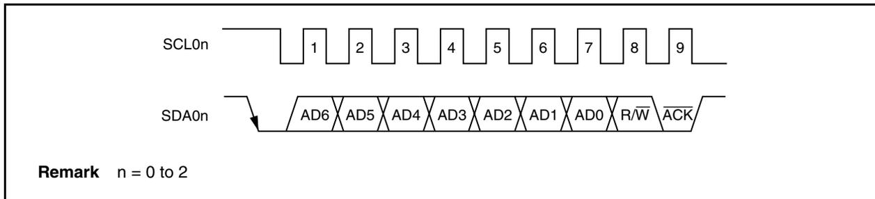
When the local address is received,  $\overline{\text{ACK}}$  is automatically generated regardless of the value of the ACKEn bit. No  $\overline{\text{ACK}}$  is generated if the received address is not a local address (NACK).
