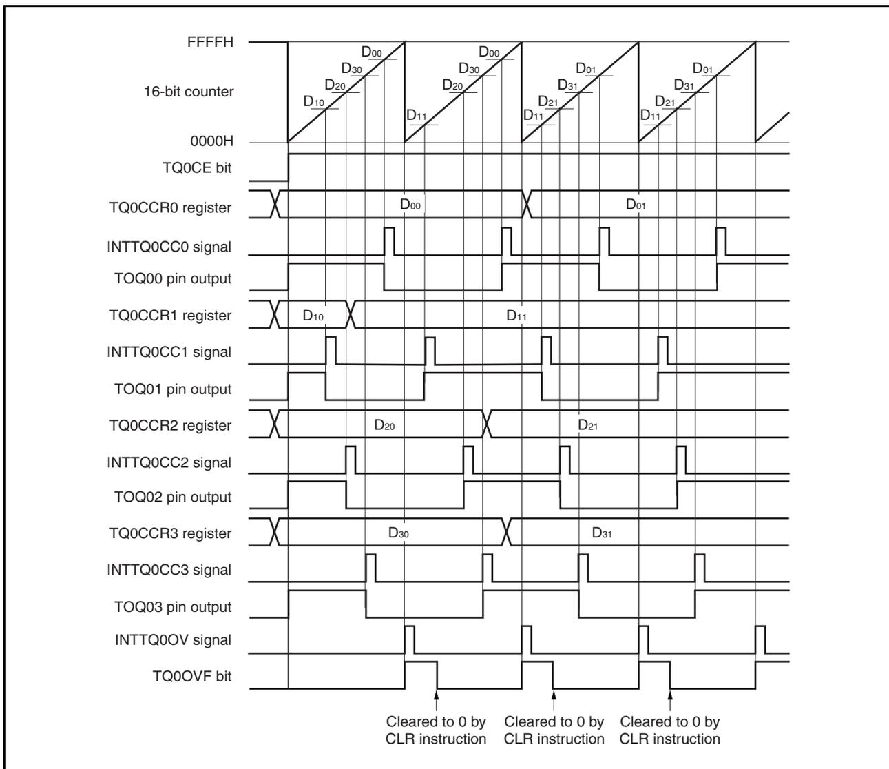
When the TQ0CE bit is set to 1, the 16-bit counter starts counting. When the valid edge input to the TIQ0m pin is detected, the count value of the 16-bit counter is stored in the TQ0CCRm register, and a capture interrupt request signal (INTTQ0CCm) is generated.
