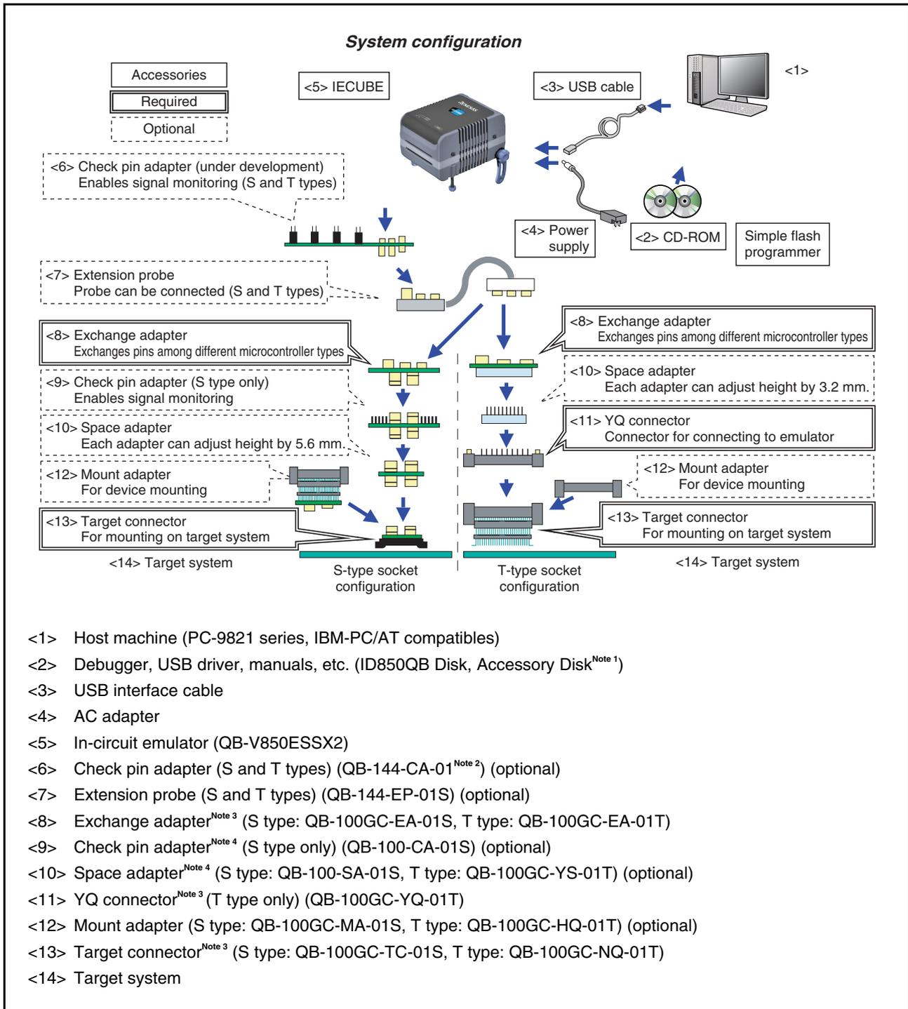
Figure A-2. System Configuration (When Using QB-V850ESSX2) (2/2)
