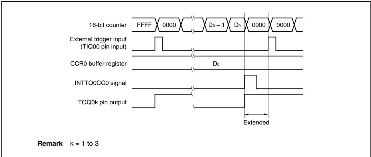
If the trigger is detected immediately before the INTTQ0CC0 signal is generated, the INTTQ0CC0 signal is not generated. The 16-bit counter is cleared to 0000H, the TOQ0k pin is asserted, and the counter continues counting. Consequently, the inactive period of the PWM waveform is shortened.
