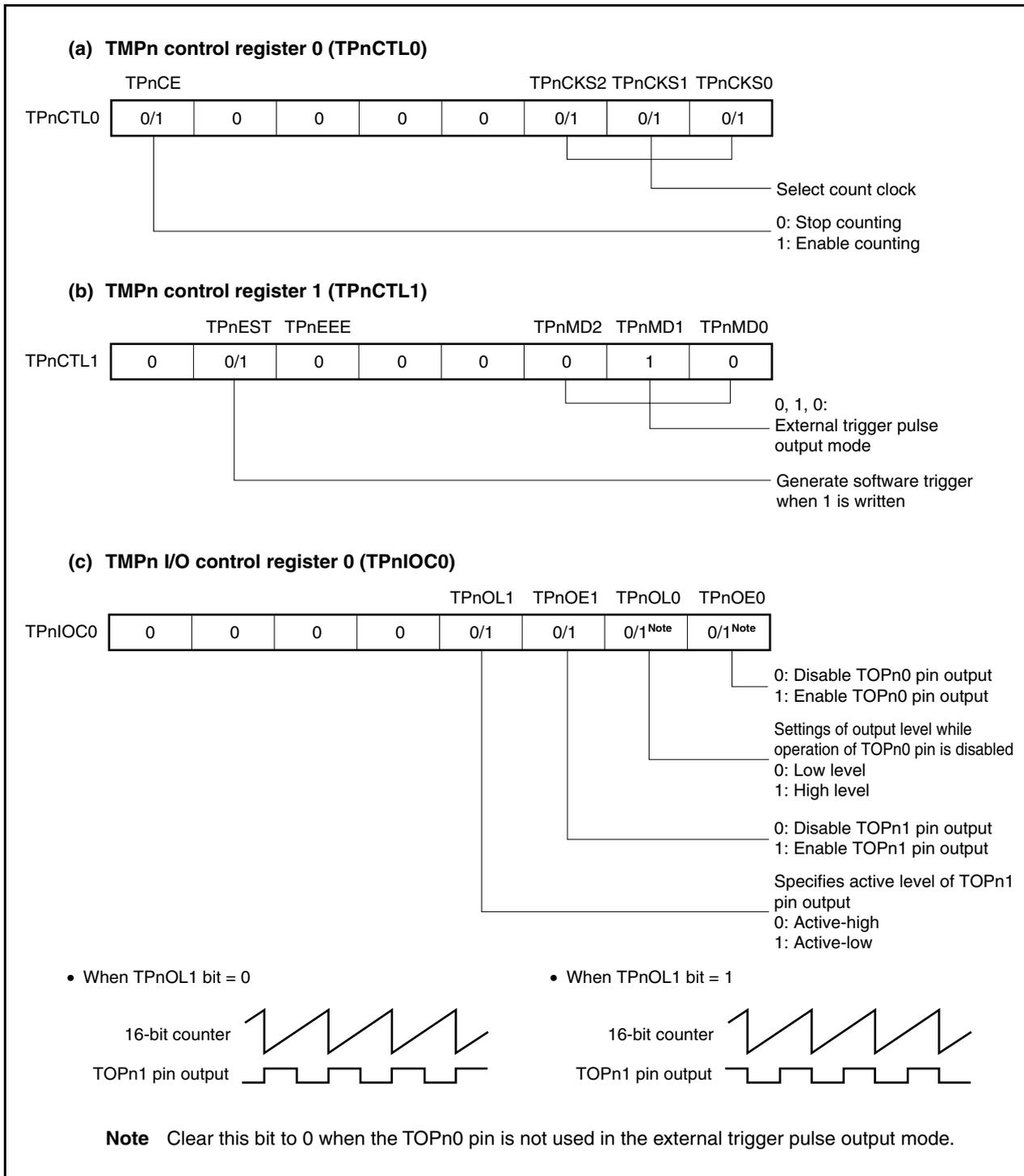
Figure 7-18. Register Setting for Operation in External Trigger Pulse Output Mode (2/2)
