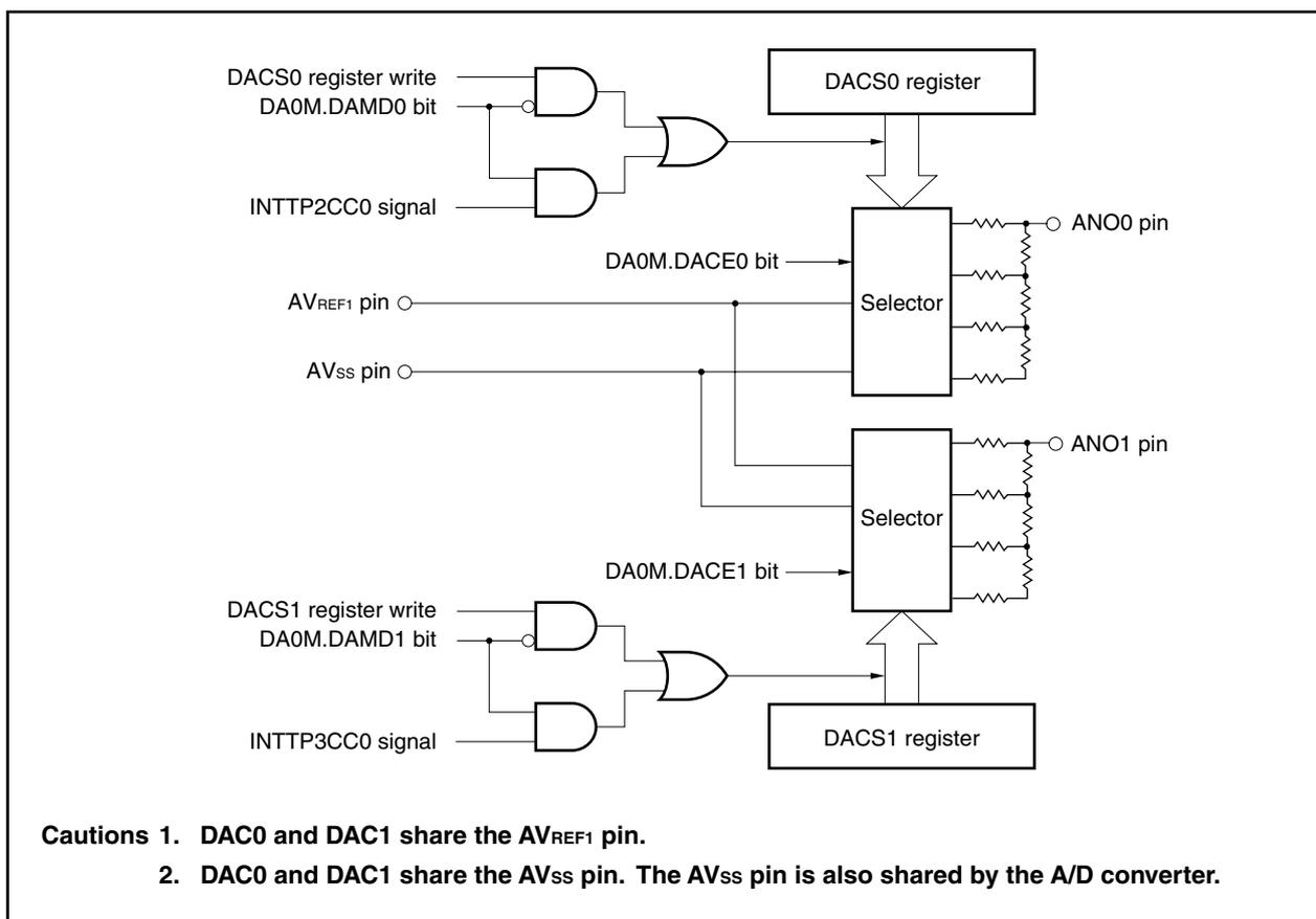
The D/A converter includes the following hardware.
