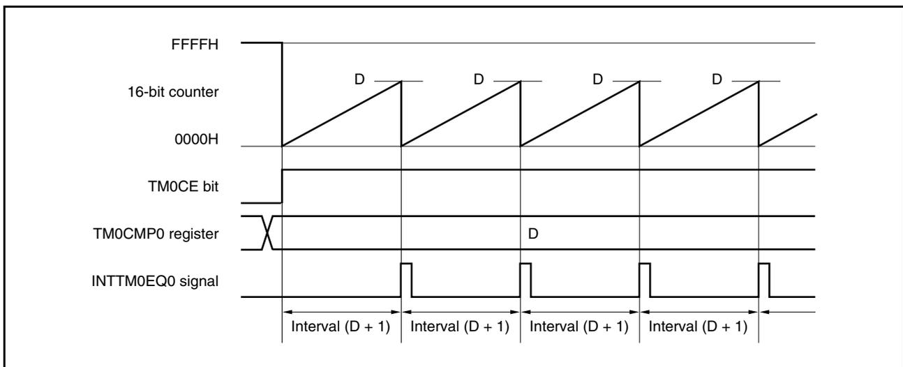
When the TM0CE bit is set to 1, the value of the 16-bit counter is cleared from FFFFH to 0000H in synchronization with the count clock, and the counter starts counting.
