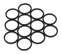
Description: These plastic shaft spacers have an inner diameter of 5/8" and a thickness of 1/16". These spacers are ideal for spacing out an area between a bearing and a shaft collar to reduce metal to metal contact.
